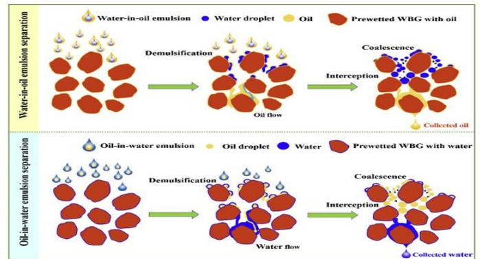
Figure 7 Oil water separation (OWE) and water oil separation (WOE) are separated using the WBG layers.
