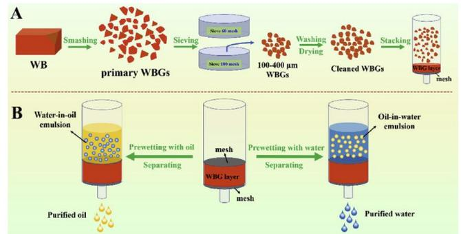
Figure 6 The preparation of green waste brick layers (A) and its application in oil-water treatment (B).
