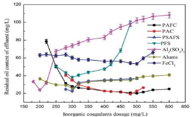
Figure 3 The influence of adding inorganic coagulant in the separation of oil and water [24]
