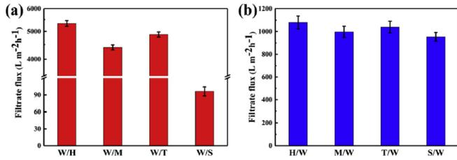
Figure 8 The diagram illustrates the filtrate fluxes versus (a) WOE and (b) OWE when the WBG layer is 3 cm thick and the solution is 10 ml in volume. [37].
