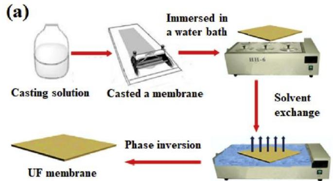
Figure 15 The schematic diagram for fabrication and enhancing UF membranes by phase inversion method
