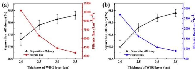
Figure 9 By increasing the WBG layer thickness, the diagram shows the separation effectiveness and filtrate flux for the W/H emulsion and the H/W emulsion, respectively. [37].
