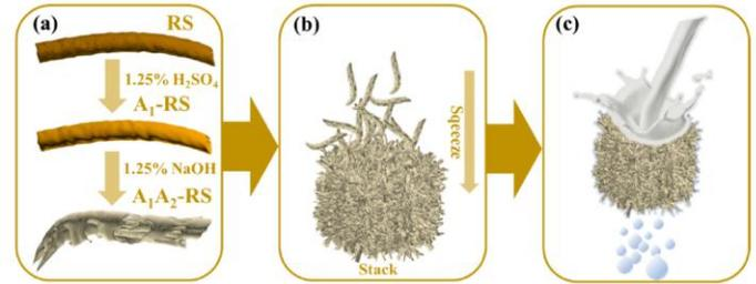
Figure 10 (a) synthesis of the A1A2-RS using a straightforward acid-base procedure; (b) Demonstrate the layer-by-layer extrusion technique. (c) the process [37]
