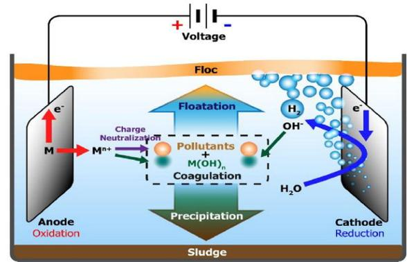
Figure 5 The electrocoagulation process' mechanism [25].
