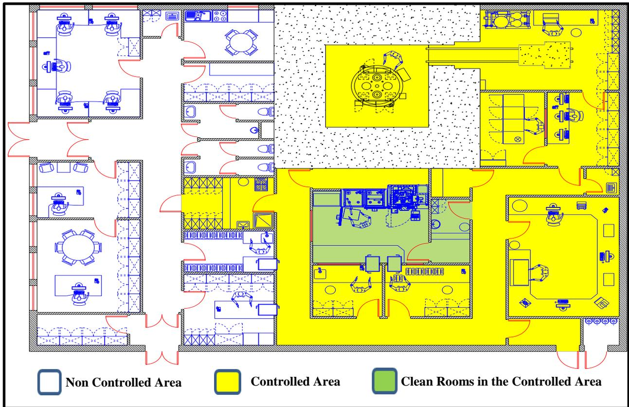
**Fig. 1:** An example of general architecture for a nuclear facility [33]
