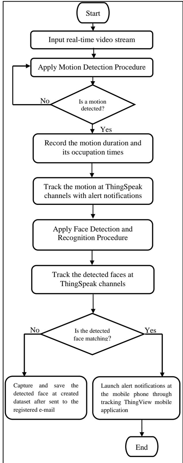
**Fig.3:** Flow chart of the moving object detection and recognition system
