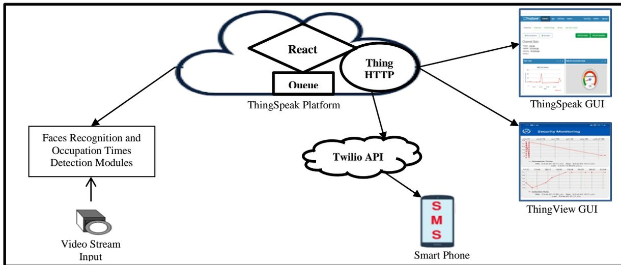
**Fig.7:** Architecture of monitoring data system with IoT
