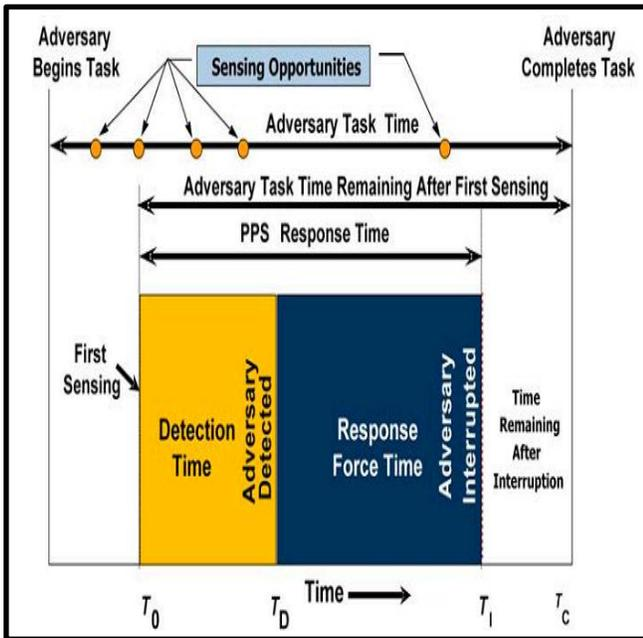
Fig. 4: The detection and response time for adversary with the physical protection system [17].
