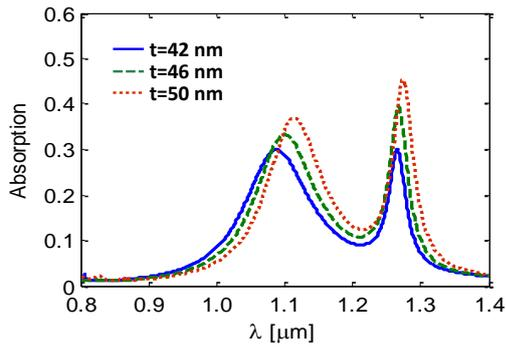
**Figure.5.** Absorption spectra of the model with variable layer thickness
