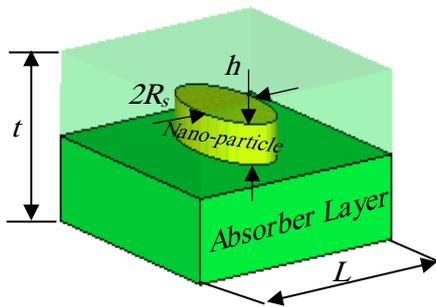
**Figure.1.** Structure of a single layer.
