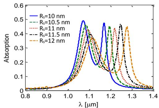
**Figure.2.** Absorption spectra of the model with various nanoparticle semi-minor axes
