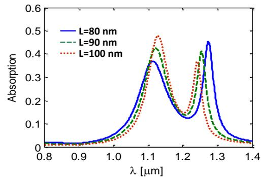
**Figure.4.** Absorption spectra of the model for several nanoparticle periodicities  $L$
