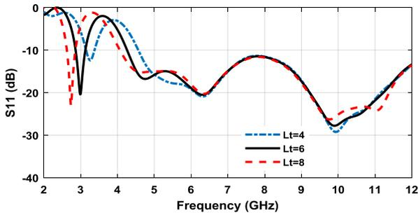
Fig. 3: Simulated S11 of the antenna with variations of the length of the radiator's slot.
