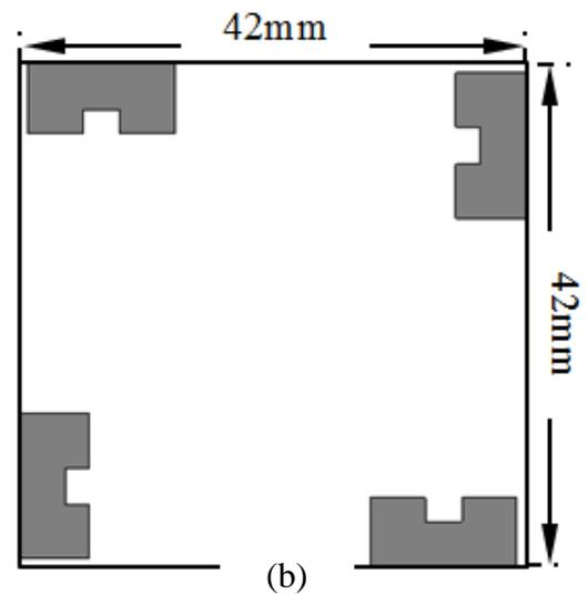
Fig. 6: Four-element MIMO antenna layout: (a) the top layer and (b) the bottom layer.
