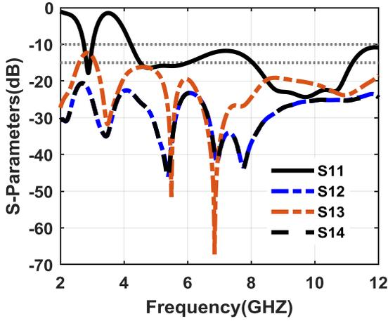
Fig.7: Simulated S-parameters of the MIMO antenna.
