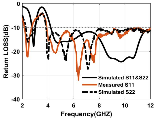
**Fig. 13:** The measured and simulated return loss of the proposed antenna.
