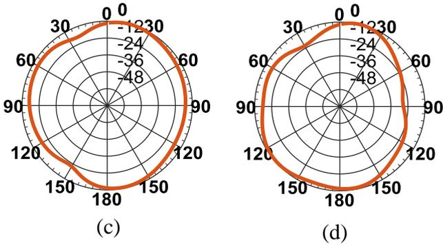
**Fig. 10:** Normalized simulated radiation pattern of the proposed antenna of Port 1: (a) x-z plane at 3.5 GHz; (b) y-z plane at 3.5 GHz; (c) x-z plane at 10 GHz; (d) y-z plane at 10 GHz.
