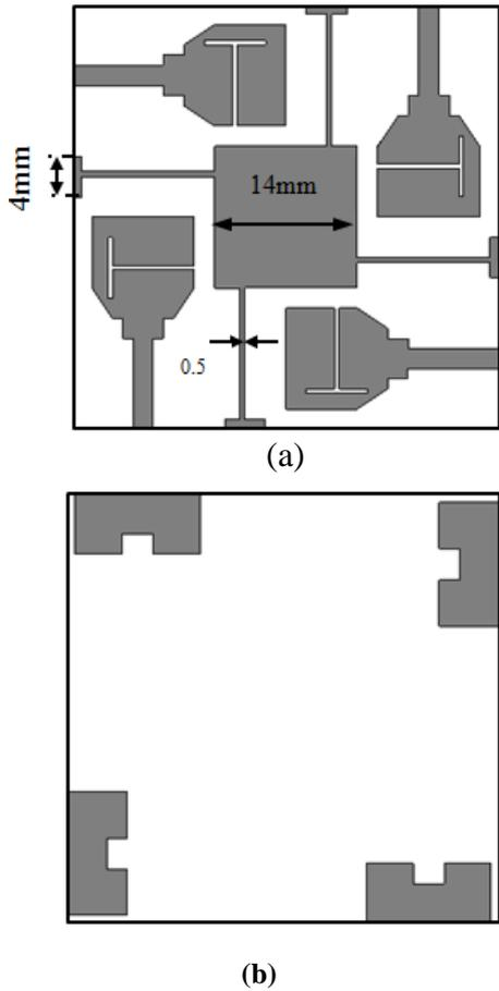
Fig. 8: Layout of the proposed antenna:(a) the top layer and (b) the bottom layer.
