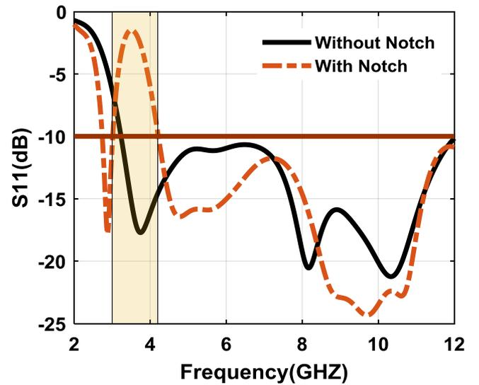
Fig. 2: The simulated return loss results of a single-element UWB antenna.
