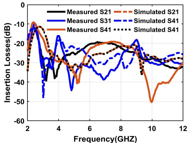
**Fig. 14:** The measured and simulated insertion of the proposed design.
