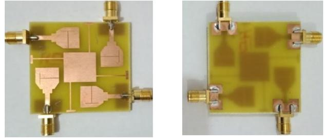
**Fig. 12:** The prototype of the proposed antenna: (a) top layer; (b) the bottom layer.
