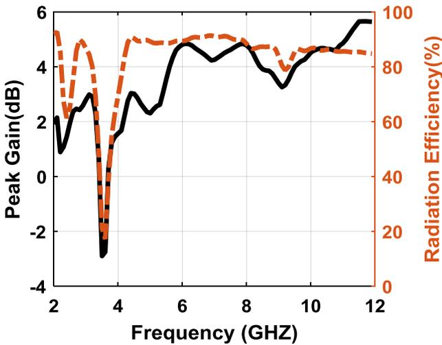
**Fig. 11:** Simulated realized peak gain and radiation efficiency of the proposed design.
