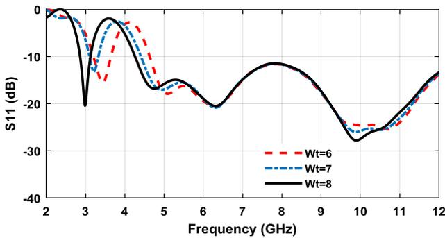
Fig. 4: Simulated S11 of the antenna with variation in the width of the radiator's slot.
