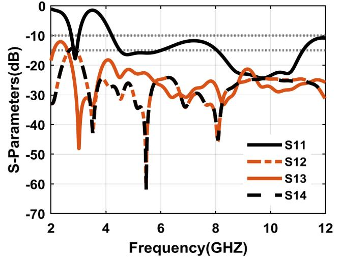
Fig.9: Simulated S-parameters of the proposed antenna.
