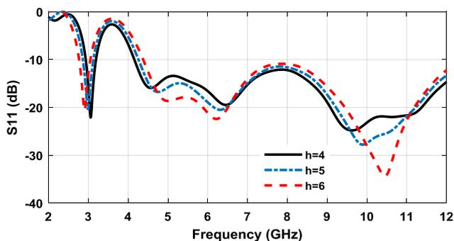
Fig. 5: Simulated S11 of the antenna with variation in the position of the radiator's slot.
