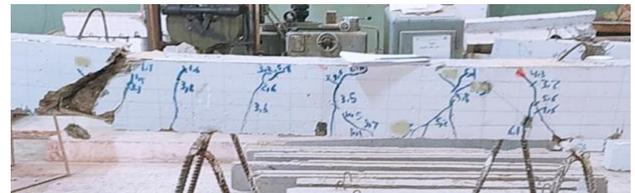
Picture.4. Mode of failure of beam (D1).
