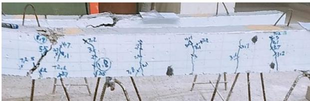
Picture.6. Mode of failure of beam (D3).
