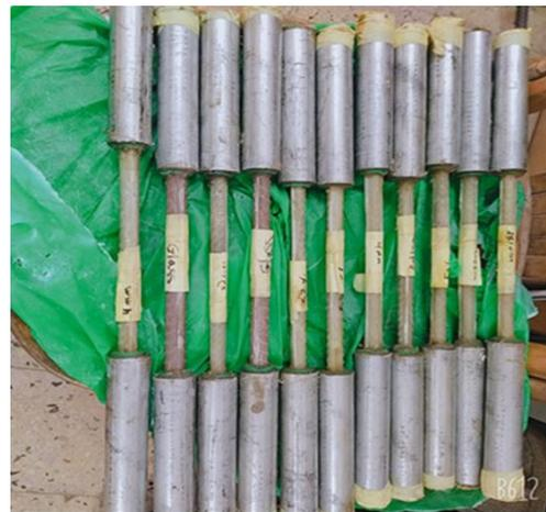
Picture.2. the Hybrid wires Bars during tension test.
