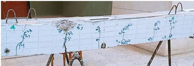
Picture.5. Mode of failure of beam (D2).
