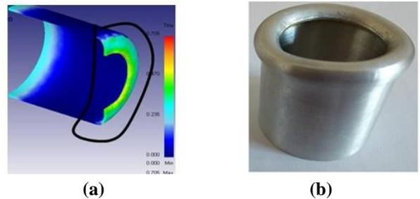
Fig. 21: Folds occurred at conical die with semi-die angle  $60^\circ$  and wall thickness 1.5 mm.
