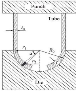
**Fig.2: Nosing process using hemispherical die Amirhosseini et al [19].**
