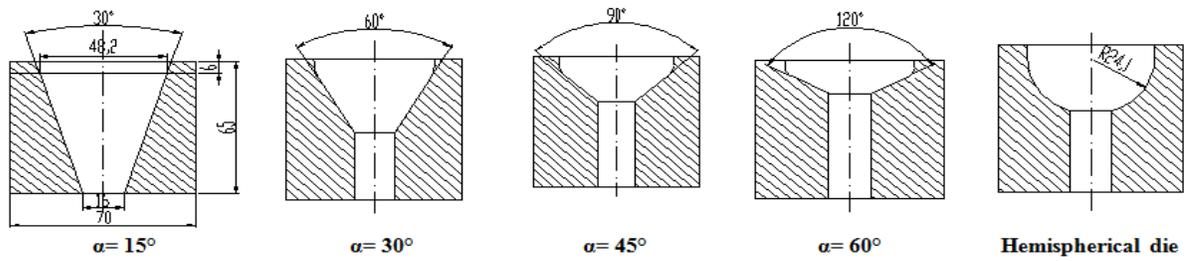
Fig.6: Schematic drawings of the tube nosing dies.
