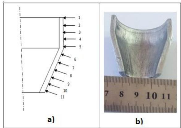
Fig. 19: a) shows the positions of thickness measurements on the nosed part b) photo of the polished sliced part at tube thickness 3.5 mm, semi-die angle  $15^\circ$ , and grease lubricated.
