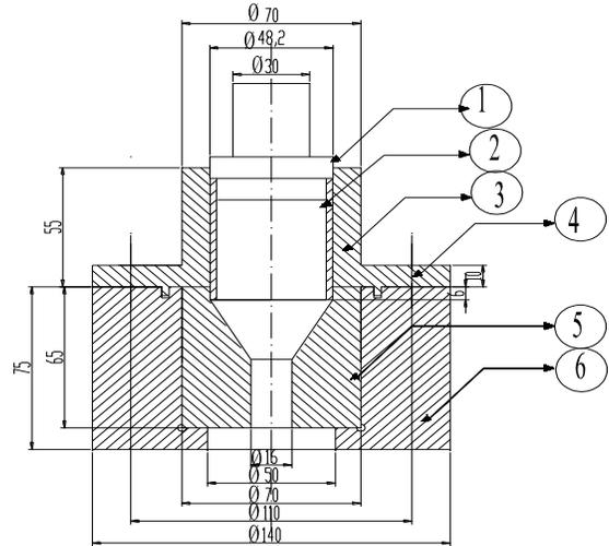
**Fig.4: Nosing setup**
