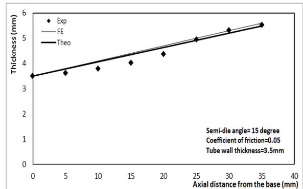
Fig. 20: Correlation between the FE-predicted and the experimentally values of thickness distribution, the values tube thickness 3.5 mm, semi-die angle  $15^\circ$ , and grease lubricated.
