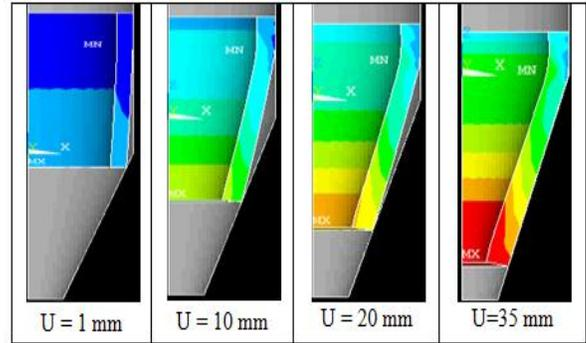
**Fig. 16 deformation shape at different die penetration at  $15^\circ$ .**
