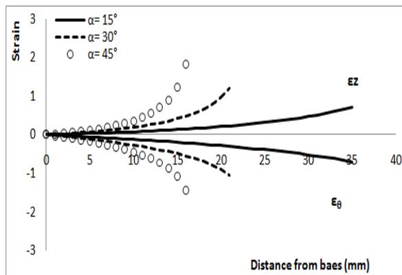
Fig.18. shows the effect of thickness strain distribution at different semi die angle.
