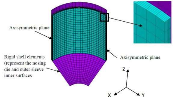
**Fig. 3: FE model showing tube and conical die for tube nosing at semi-die angle 15 degree.**
