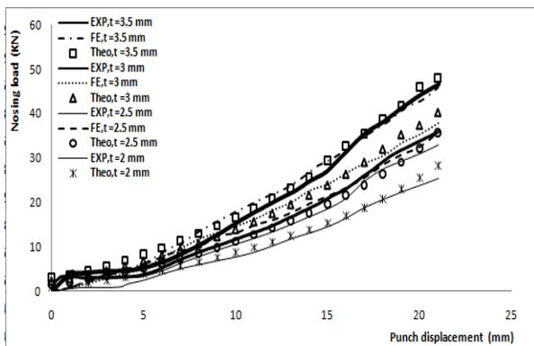
Fig.9a. load/ displacement curve at  $\alpha=30^\circ$ , and  $\mu=0.15$ .
