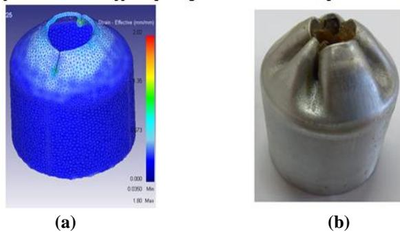
**Fig. 22: Wrinkling at conical semi-die angle 45°, wall thickness 1mm and grease-lubricated.**
