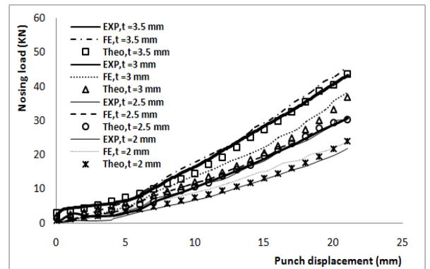
Fig.9c. load/ displacement curve at  $\alpha=30^\circ$ , and  $\mu=0.04$ .
