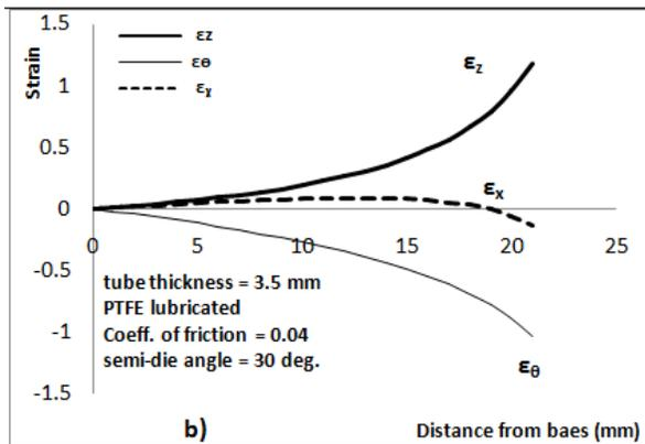
Fig.17. Strain distribution of nosed tube:
