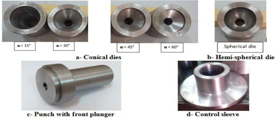
Fig. 7: Photos of manufactured dies, new designed plunger punch and control sleeve design.
