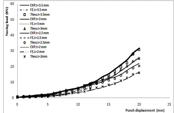
Fig.12 load/ displacement curve in hemispherical die at  $\mu=0.05$ .
