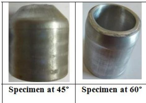
Fig.11 the deformed tubes after nosing process.
