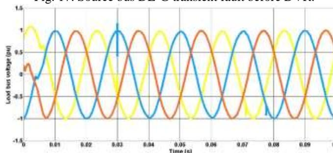
Fig. 18. Load bus voltage after DVR.
