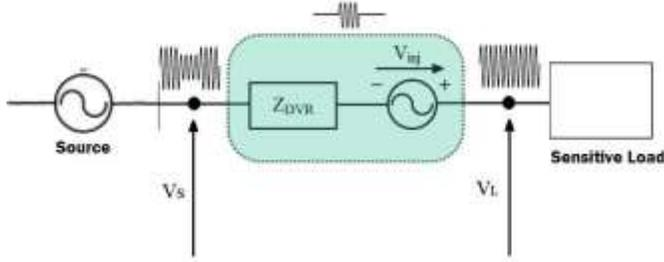
Fig. 5. DVR equivalent circuit diagram.
