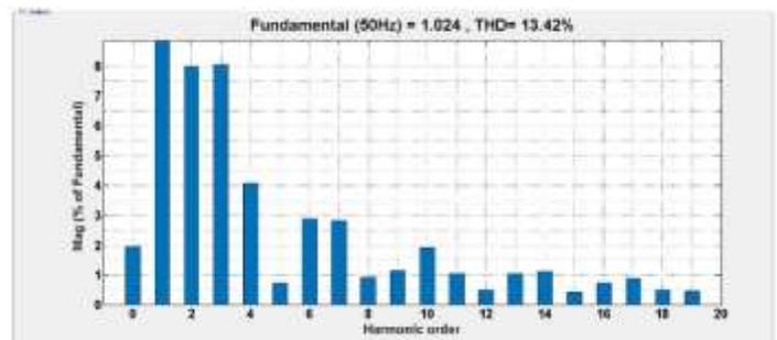
Fig. 15. THD of source bus voltage before DVR
