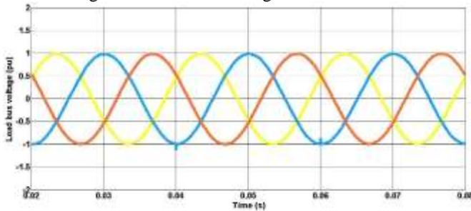
Fig. 12. Load bus voltage after DVR.
