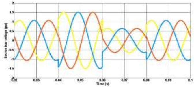
Fig. 13. Source bus voltage fluctuation before DVR.
