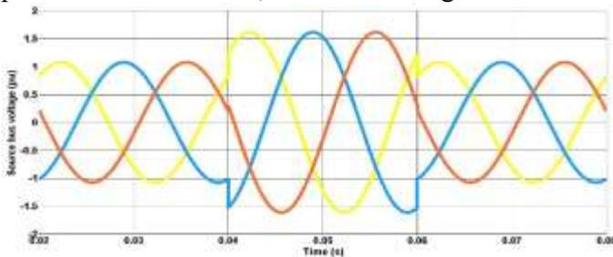
Fig. 11. Source bus voltage swell before DVR.
