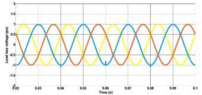
Fig. 14. Load bus voltage after DVR.
