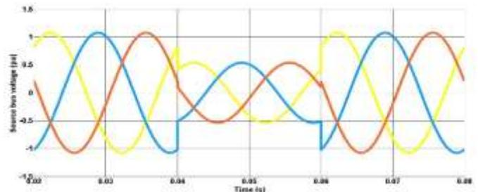
Fig. 9. Source bus voltage sag before DVR.
