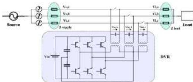
Fig. 6. Two-level converters DVR topology.
