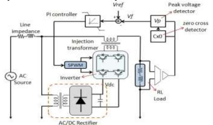
Fig. 7. Design of Two-level inverter DVR.
