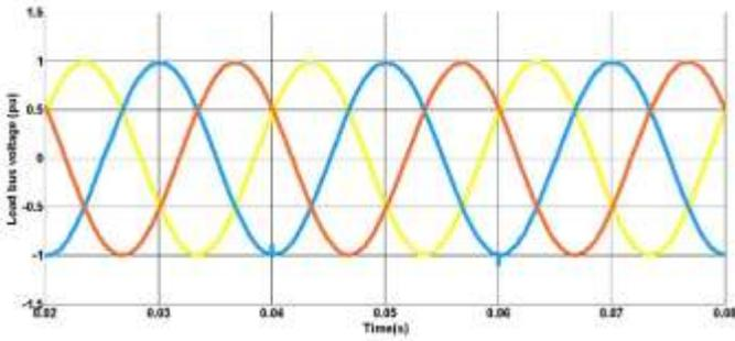
Fig. 10. Load bus voltage after DVR.
