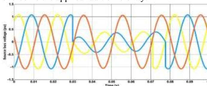
Fig. 17. Source bus DL-G transient fault before DVR.
