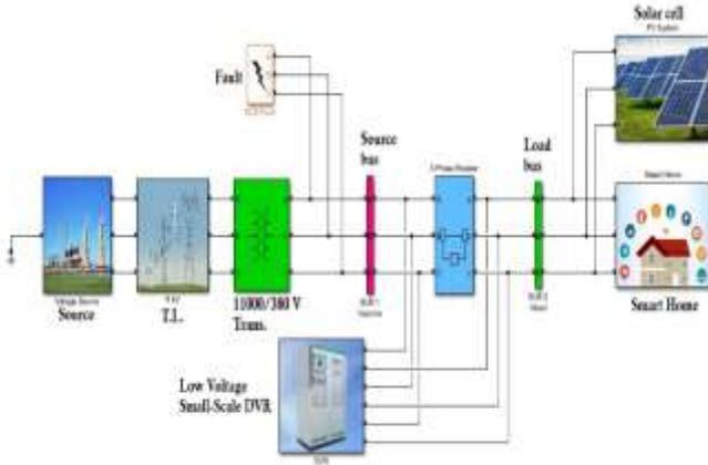
Fig. 8. Low-Cost Two-level inverter DVR with a smart home-smart grid model.
