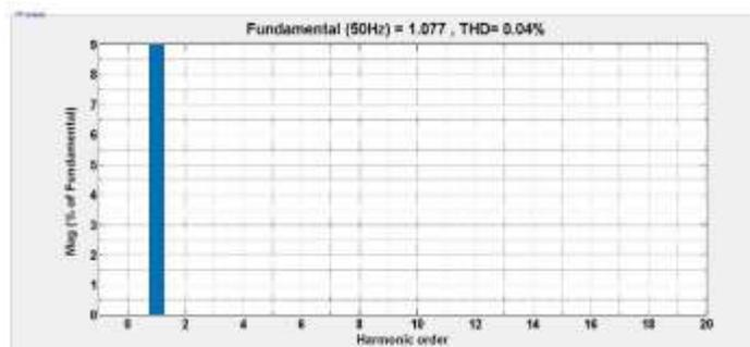
Fig. 16. THD of load bus voltage after DVR.
