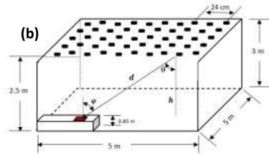
**Fig. 1.** Room configuration for (a) distinctive lighting layout, (b) uniform lighting layout.
