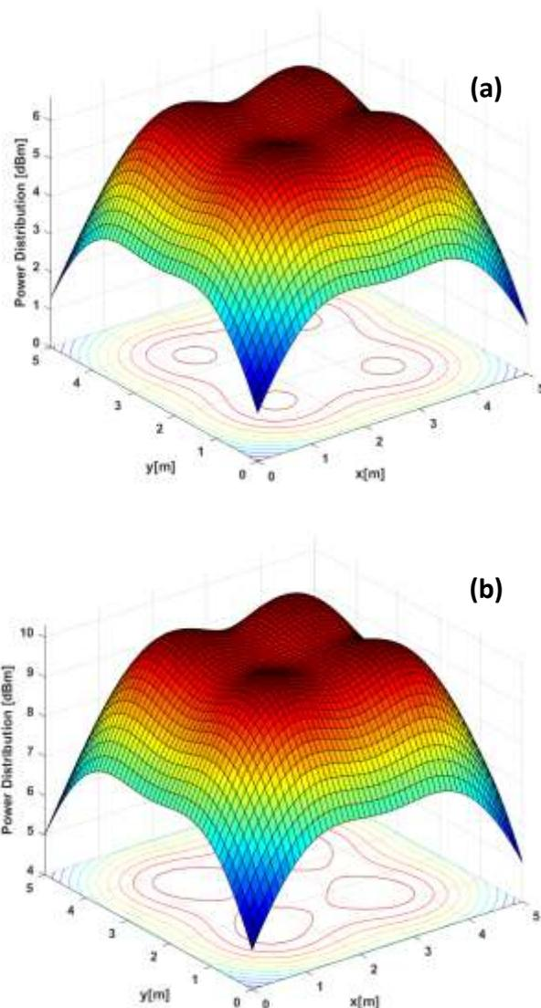
**Fig. 8** Power distribution across the proposed room under distinctive lighting topology assumption for SC- LPPM (a) without utilizing OFDM techniques, (b) by utilizing OFDM techniques.
