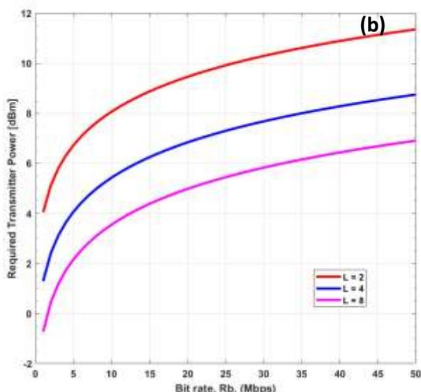
**Fig. 7** Minimum transmitter power required vs. bit rate at different modulation levels ( $L$ ) under uniform lighting topology assumption for (a) without utilizing OFDM techniques, (b) by utilizing OFDM techniques.
