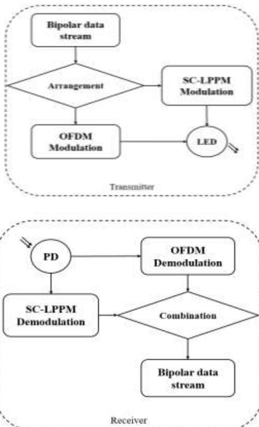
Fig. 3. Block diagram for the proposed
