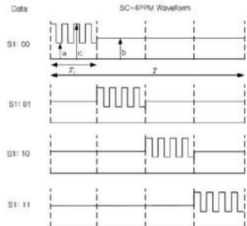
**Fig. 2.** SC-4 PPM waveform [21, 35].
