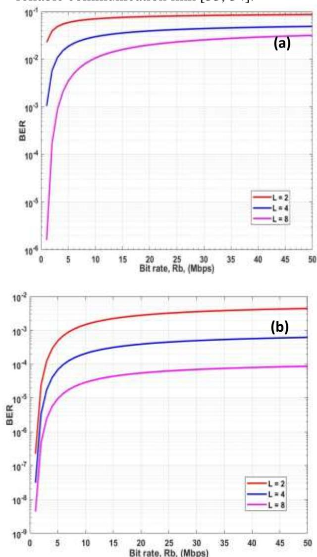
Fig. 4 BER vs. bit rate at different modulation levels ( $L$ )
