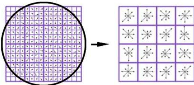
**Fig. 4:** Mechanism of the SIFT features for a 16x16 pixel and a 4x4 array.
