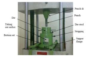
Figurel: Developed deep drawing apparatus.
