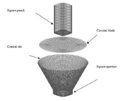
Figure 4: FEM mesh of square punch, conical die, and circular blank.
