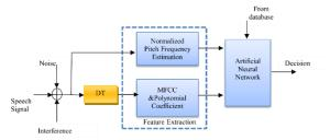
(b) Testing phase of the proposed ASI system in the presence of interference.
