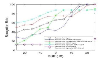
Figure 11: Recognition rate versus SNR for the ASI system on speech signals contaminated by AWGN and interference with a preprocessing wavelet hard thresholding stage (single-level Haar wavelet).
