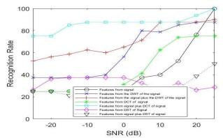
Figure 7: Recognition rate versus SNR for the ASI system on speech signals contaminated by AWGN and interference with a preprocessing adaptive Wiener filtering stage.
