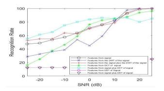
Figure 9: Recognition rate versus SNR for the ASI system on speech signals contaminated by AWGN and interference with a preprocessing wavelet hard thresholding stage (single-level Daubechies wavelet)
