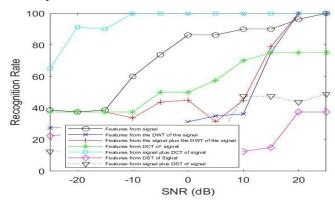
**Figure 12**: Recognition rate versus SNR for the ASI system on speech signals contaminated by AWGN and interference with a preprocessing wavelet soft thresholding stage (two-level Daubechies wavelet).
