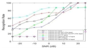
Figure 8: Recognition rate versus SNR for the ASI system on speech signals contaminated by AWGN and interference with a preprocessing wavelet soft thresholding stage (single-level Daubechies wavelet).
