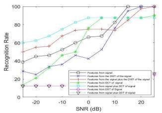
**Figure 10**: Recognition rate versus SNR for the ASI system on speech signals contaminated by AWGN and interference with a preprocessing wavelet soft thresholding stage (single-level Haar wavelet).
