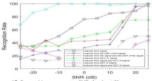
**Figure.15**: Recognition rate versus SNR for the ASI system on speech signals contaminated by AWGN and interference with a preprocessing wavelet hard thresholding stage (two-level Haar wavelet).
