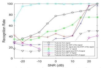
speech signals contaminated by AWGN and interference with a preprocessing wavelet hard thresholding stage (two-level Daubechies wavelet).
