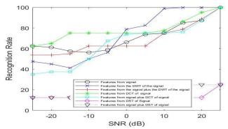
Figure 6: Recognition rate versus SNR for the ASI system on speech signals contaminated by AWGN and interference with a preprocessing Wiener filtering stage.
