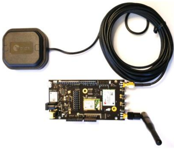
Figure 3 GPS receiver board and its U-Blox multi-band GNSS antenna.
