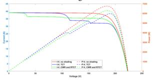
Figure 10. (I-V) and (P-V) characteristic curves of the PV system under shading pattern No. 2
