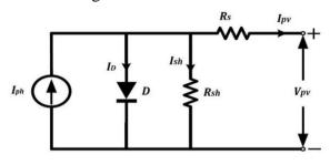
Figure 1. Single diode model
