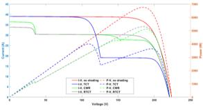
Figure 9. (I-V) and (P-V) characteristic curves of the PV system under shading pattern No. 1
