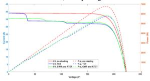
Figure 11. (I-V) and (P-V) characteristic curves of the PV system under shading pattern No. 3
