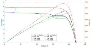
Figure 13. (I-V) and (P-V) characteristic curves of the PV system under shading pattern No. 5
