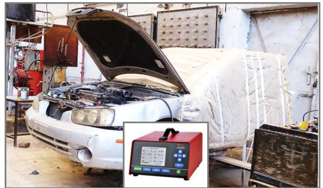
Figure 4: Instrumentation setup of A/C system of vehicle
