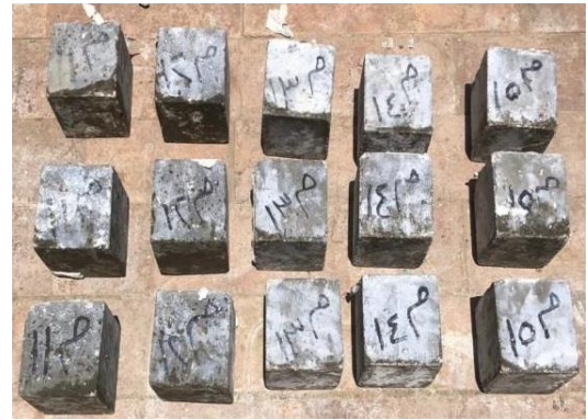
Figure 4: Specimen after pouring
