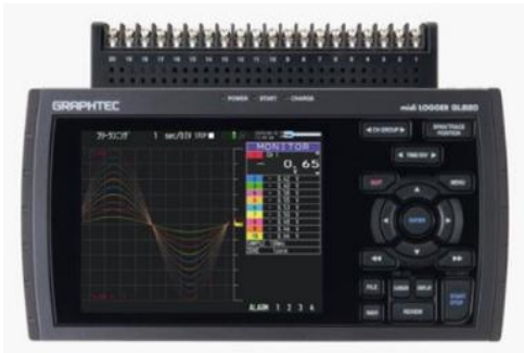
Figure 5: Data store and transfer unit to the computer (midi LOGGER GL820)
