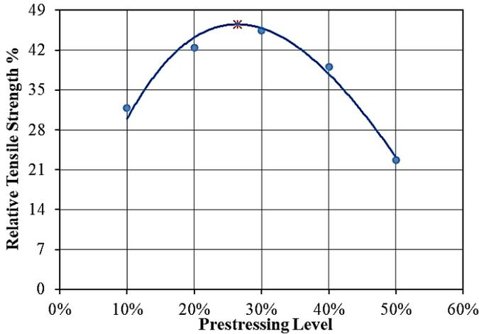
Figure 14: Variation of the relative tensile strength of the PGFRP with prestressing levels
