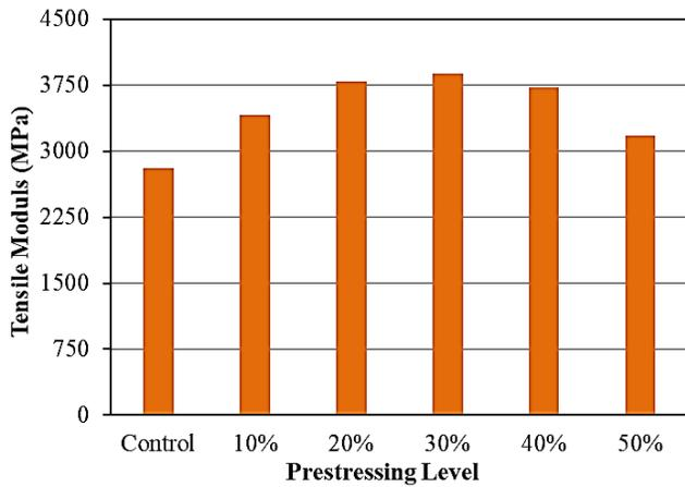
**Figure 11: Variation of the tensile modulus of the PGFRP with prestressing levels**
