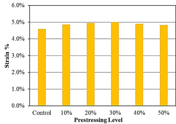
**Figure 13: Variation of the fracture strain of the PGFRP with prestressing levels**
