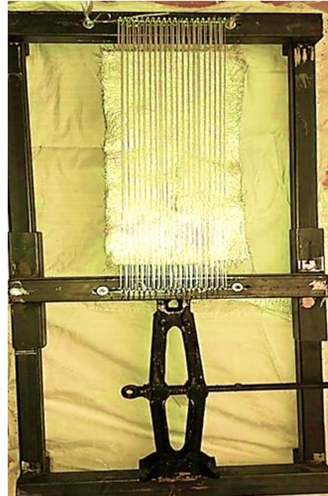
Figure 2: Image showing the uniaxial prestressing test rig used to prepare the PGFRP laminates
