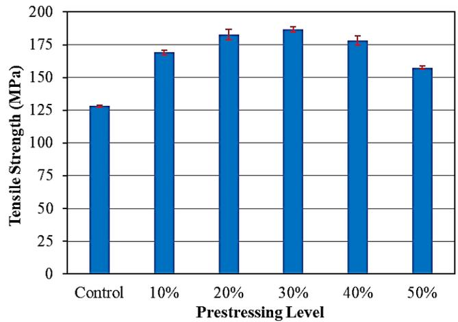
**Figure 10: Variation of the tensile strength of the PGFRP with prestressing levels**
