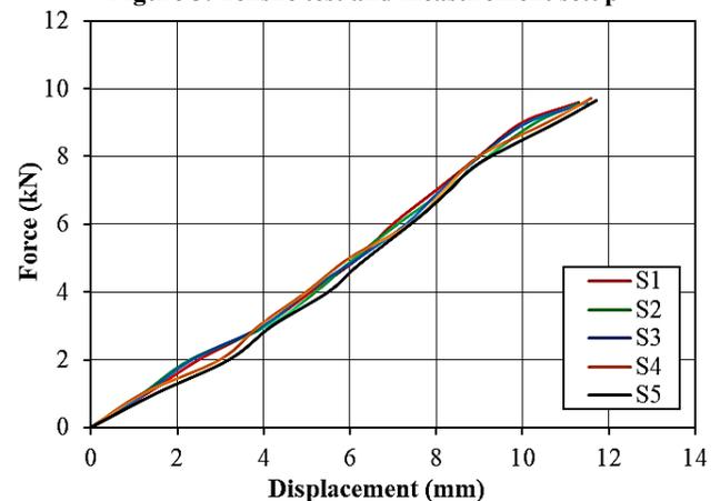
Figure 6: The relationship between applied load and displacement for five control specimens, labeled S1 to S5
