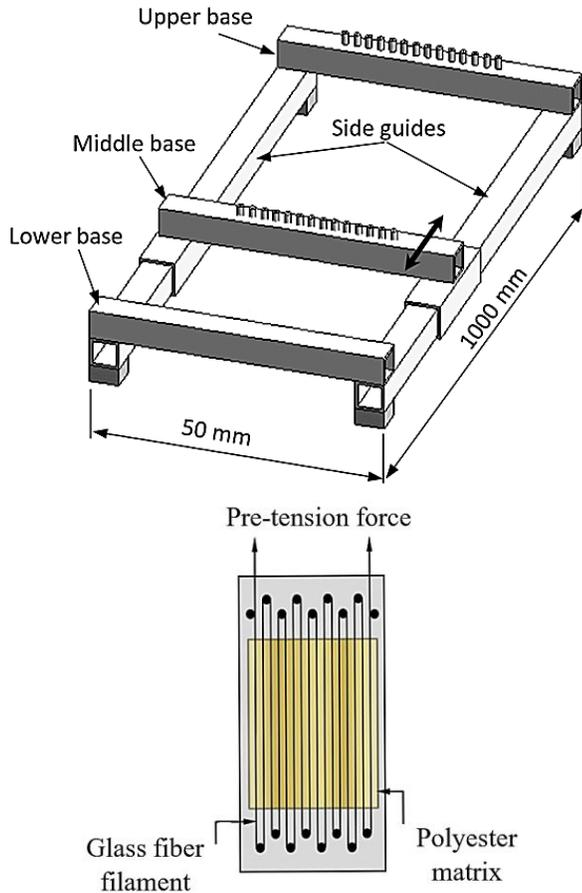
Figure 1: Schematic of the uniaxial fiber prestressing test rig
