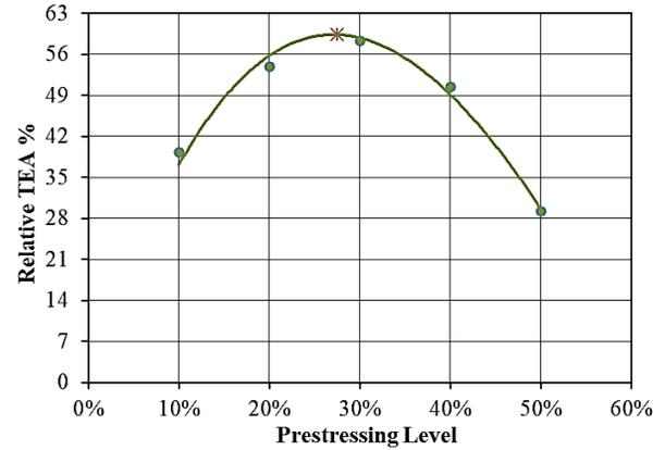
Figure 16: Variation of the relative TEA of the PGFRP with prestressing levels
