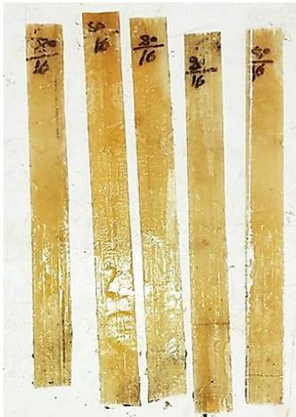
Figure 4: Manufactured prestressed glass fiber reinforced polyester composite test specimens
