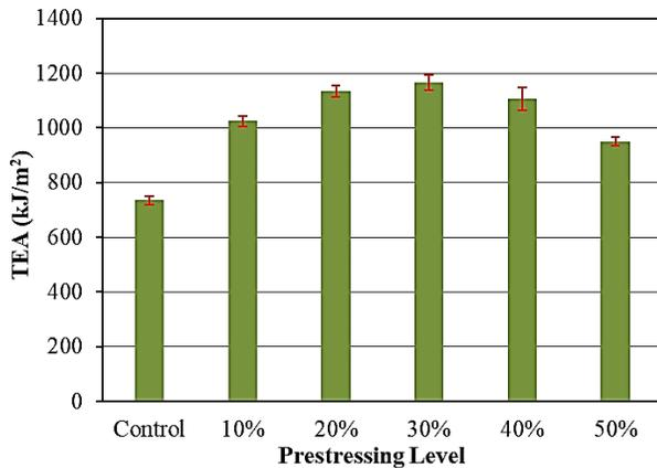
**Figure 12: Variation of the TEA of the PGFRP with prestressing levels**
