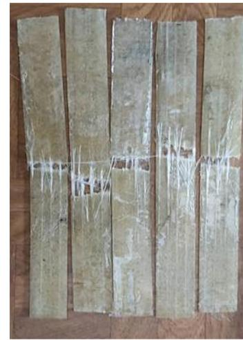
**Figure 9: The failure mode of the tested PGFRP specimens**
