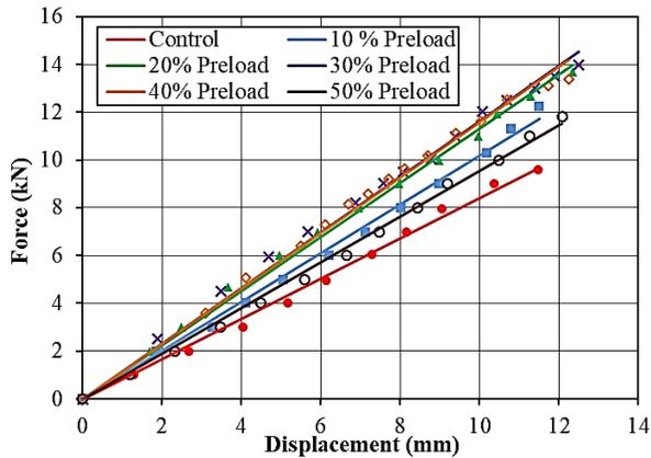
**Figure 8: Variation of the average force and average displacement for different prestressing levels**
