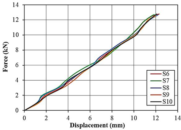
**Figure 7: The relationship between applied load and displacement for five 10% prestressing level specimens, labeled S6 to S10**
