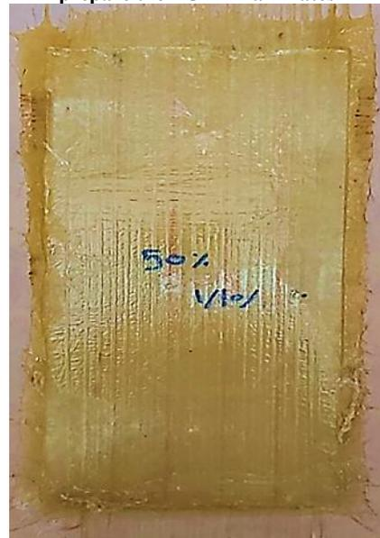
Figure 3: Manufactured prestressed glass fiber reinforced polyester composite laminate
