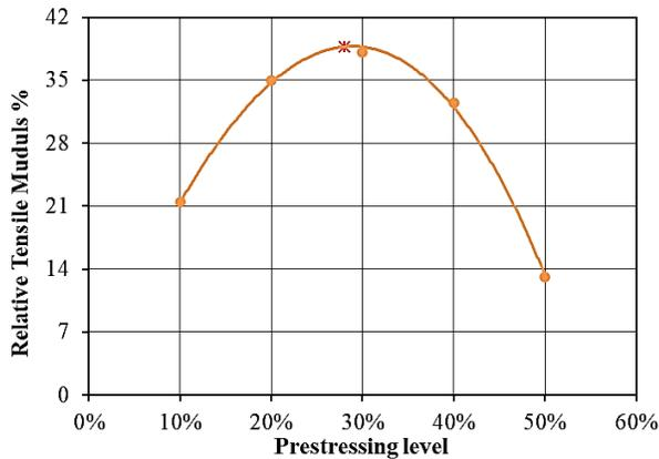
Figure 15: Variation of the relative tensile modulus of the PGFRP with prestressing levels
