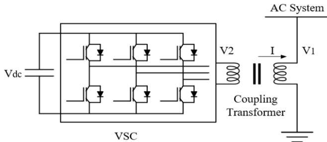
Figure 1: STATCOM's basic arrangement
