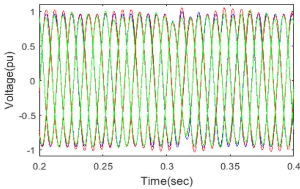
**Figure 33: The pattern of voltage waves on the B1 bus without, with STATCOM-PI controller and STATCOM-FLC under single-phase grounding fault within load A introduced at  $t = (0.3-0.31)$  seconds**
