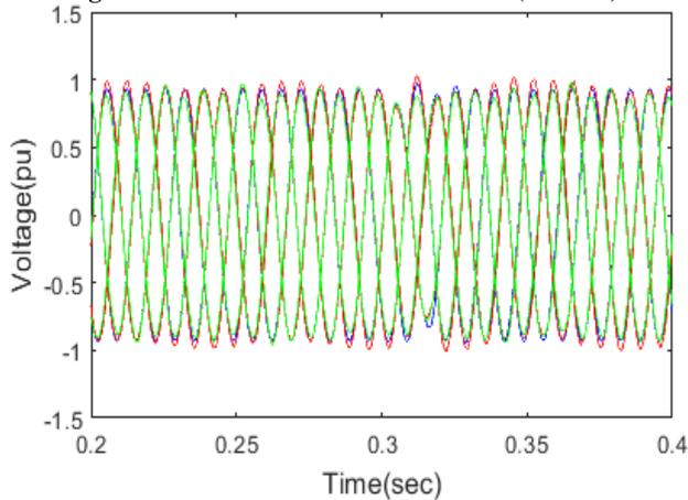
**Figure 34: The pattern of voltage waves on the B5 bus without, with STATCOM-PI controller and STATCOM-FLC under single-phase grounding fault within load A introduced at  $t = (0.3-0.31)$  seconds**
