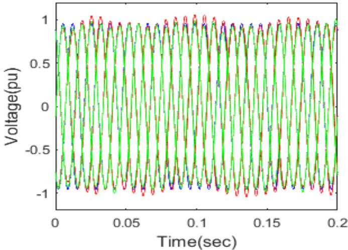
Figure 19: The pattern of voltage waves on the B1 bus without, with STATCOM-PI controller and STATCOM-FLC under standard operation
