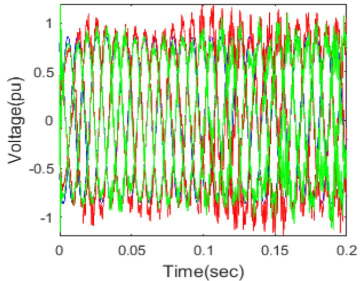
Figure 21: The pattern of voltage waves on the B11 bus without, with STATCOM-PI controller and STATCOM-FLC under standard operation
