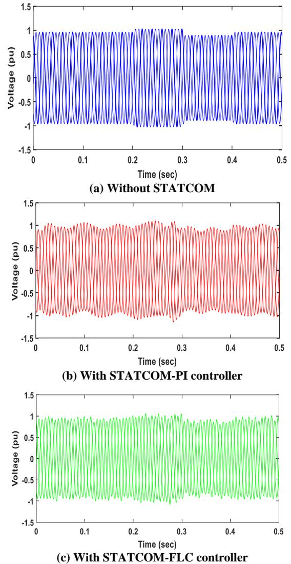
**Figure 8: The patterns of voltage waves on the B1 bus without, with STATCOM-PI controller and STATCOM-FLC under standard operation**
