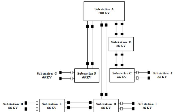
**Figure 4: The block diagram of electrical power transmission substations in Middle Egypt Electricity Zone under study**
