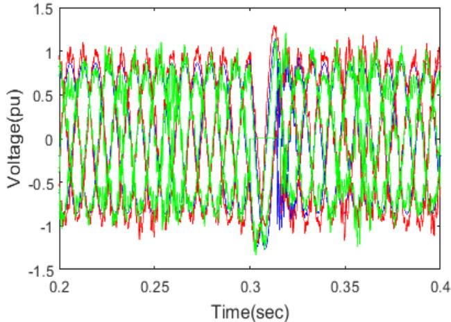
**Figure 34b: The pattern of voltage waves on the B11 bus without, with STATCOM-PI controller and STATCOM-FLC under single-phase grounding fault within load A introduced at  $t = (0.3-0.31)$  seconds**
