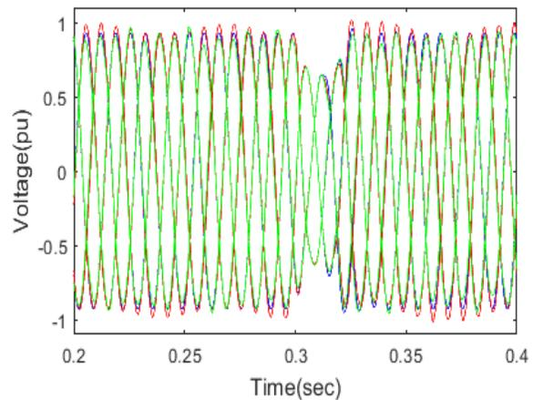
**Figure 47:** The pattern of voltage waves on the B5 bus without, with STATCOM-PI controller and STATCOM-FLC under three-phase grounding fault within load A introduced at  $t = (0.3-0.31)$  seconds
