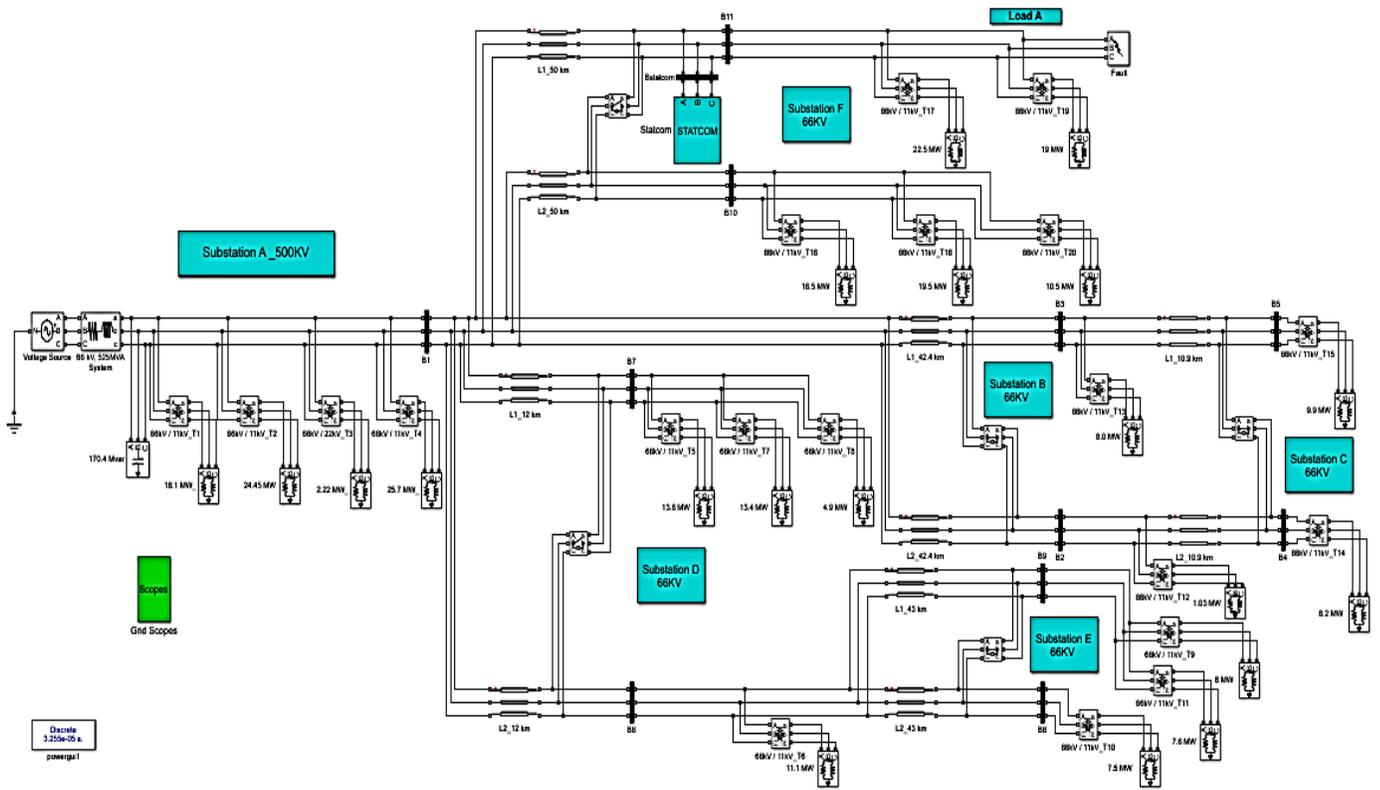
Figure 5: The proposed model of the electrical transmission network in MATLAB/Simulink
