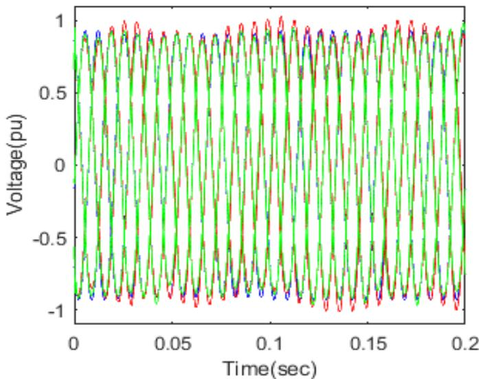
Figure 20: The pattern of voltage waves on the B5 bus without, with STATCOM-PI controller and STATCOM-FLC under standard operation
