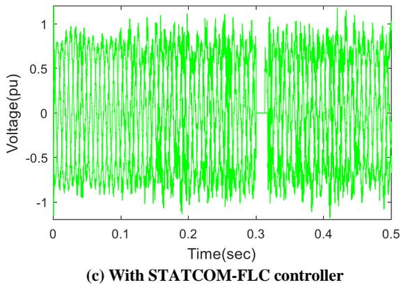
**Fig. 45:** The patterns of voltage waves on the B11 bus without, with STATCOM-PI controller and STATCOM-FLC under three-phase to ground fault within load A introduced at  $t = (0.3-0.31)$  seconds
