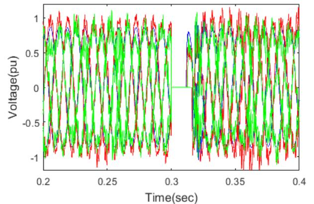
**Figure 48:** The pattern of voltage waves on the B11 bus without, with STATCOM-PI controller and STATCOM-FLC under three-phase grounding fault within load A introduced at  $t = (0.3-0.31)$  seconds
