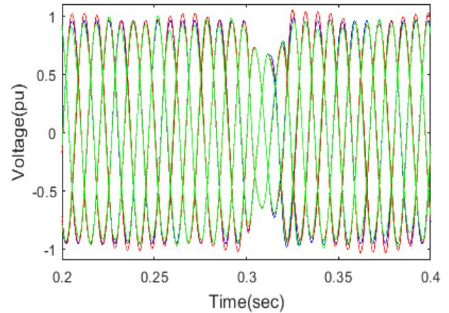
**Figure 46:** The pattern of voltage waves on the B1 bus without, with STATCOM-PI controller and STATCOM-FLC under three-phase grounding fault within load A introduced at  $t = (0.3-0.31)$  seconds
