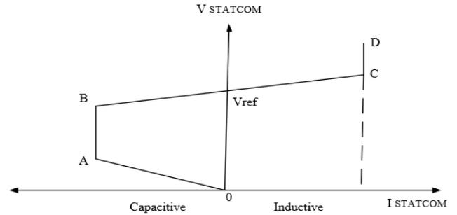
Figure 2: Voltage-Current characteristics of STATCOM
