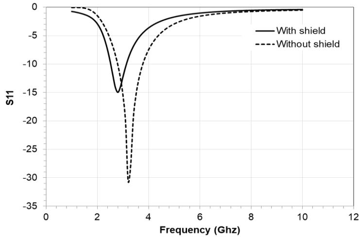
Fig.10 :Comparison of the input returns loss (S11) versus frequency of LNA circuit with and without PGS.
