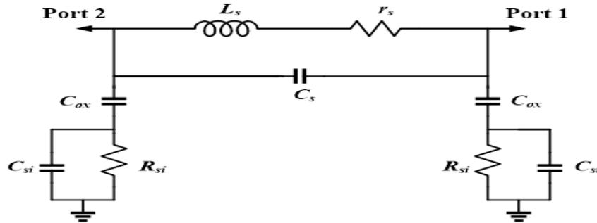
Fig. 1: Lumped model of a spiral inductor
