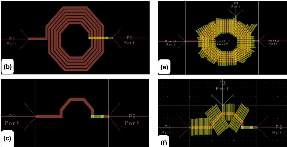
**Fig.3 :** (a) layout of the The inductive load (L3), (b) layout of the The matching inductor (L4), (c):layout of The source degeneration inductor (L2), (d): layout of the the inductive inductor with PGS, (e): layout of the matching inductor with PGS, (f): layout of The source degeneration inductor with PGS.
