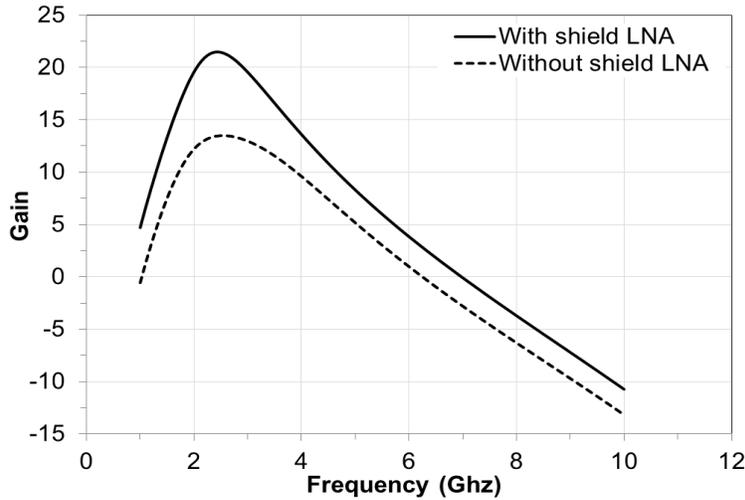
Fig.8 : Comparison of the Gain (S21) versus frequency of LNA circuit with and without PGS.
