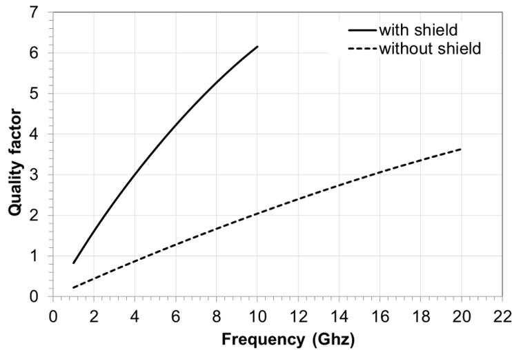
Fig.6 : Comparison of the Q-factor versus frequency of The source degeneration inductor with and without PGS.
