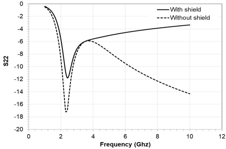
Fig.11 :Comparison of the output return loss (S22) versus frequency of LNA circuit with and without PGS.
