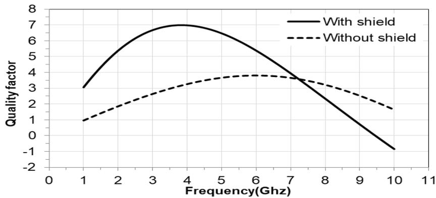
**Fig.4 :** Comparison of the Q-factor versus frequency of inductive inductor with and without PGS.
