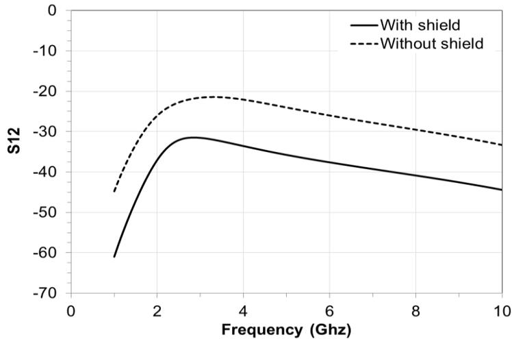
Fig.9 : Comparison of the reverse isolation (S12) versus frequency of LNA circuit with and without PGS.
