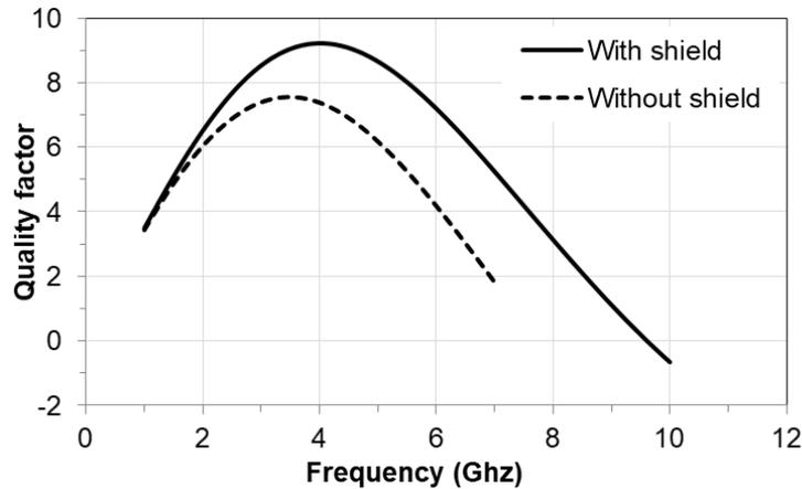
Fig.5 : Comparison of the Q-factor versus frequency of matching inductor with and without PGS.
