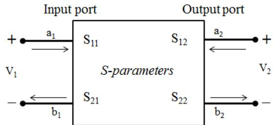
Fig.7 : Schematic block of a two-port network system.
