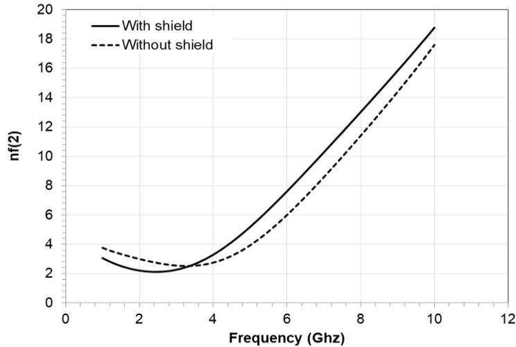
Fig.12 :Comparison of the minimum noise figure nf(2) versus frequency of LNA circuit with and without PGS.
