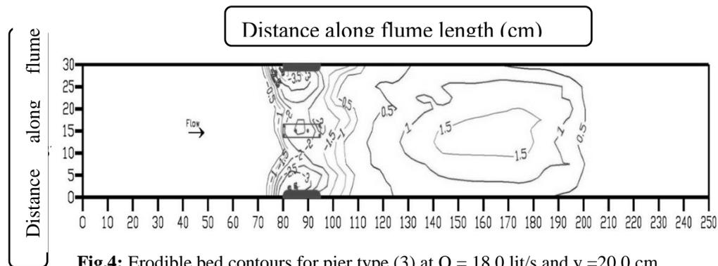
**Fig.4:** Erodible bed contours for pier type (3) at  $Q = 18.0$  lit/s and  $y = 20.0$  cm.
