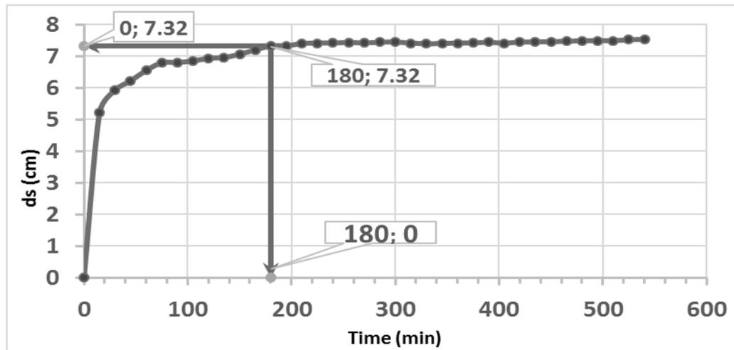
Fig.2. Equilibrium time at  $Q = 18.0$  l/s and  $y = 18.0$  cm in case oblong pier without slots.
