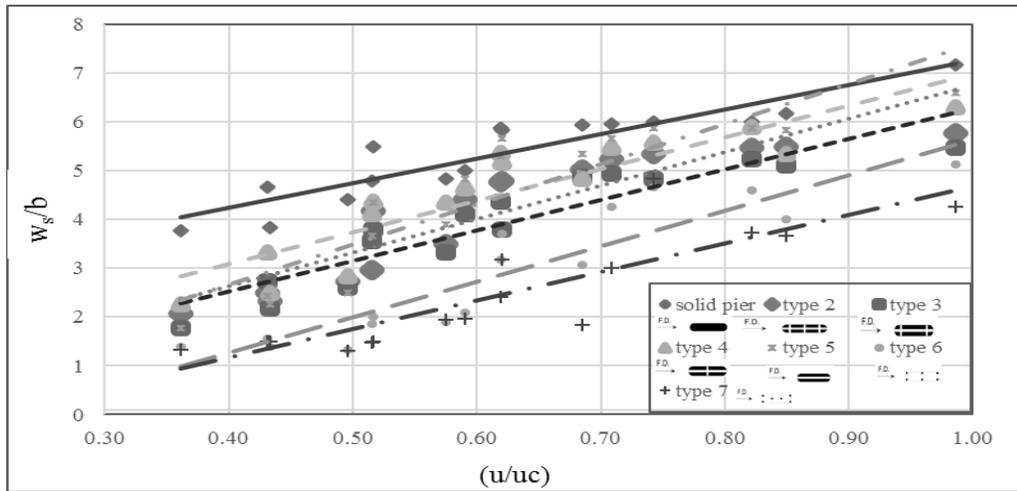
**Fig.12.** Values of relative scour hole width ( $w_s/b$ ) versus ( $u/u_c$ ) for different pier types.
