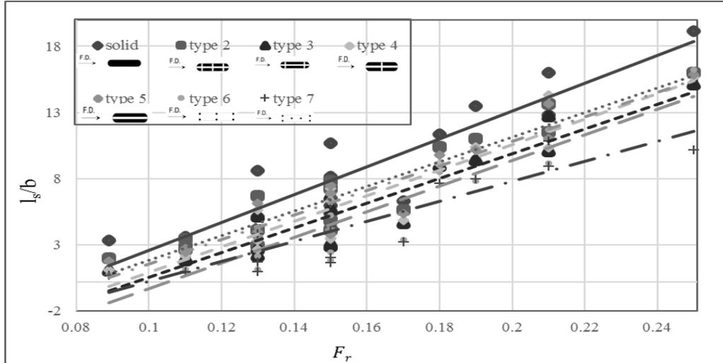
**Fig.10.** Values of relative scour hole length ( $l_s/b$ ) versus Froud number ( $F_r$ ) for different pier types.
