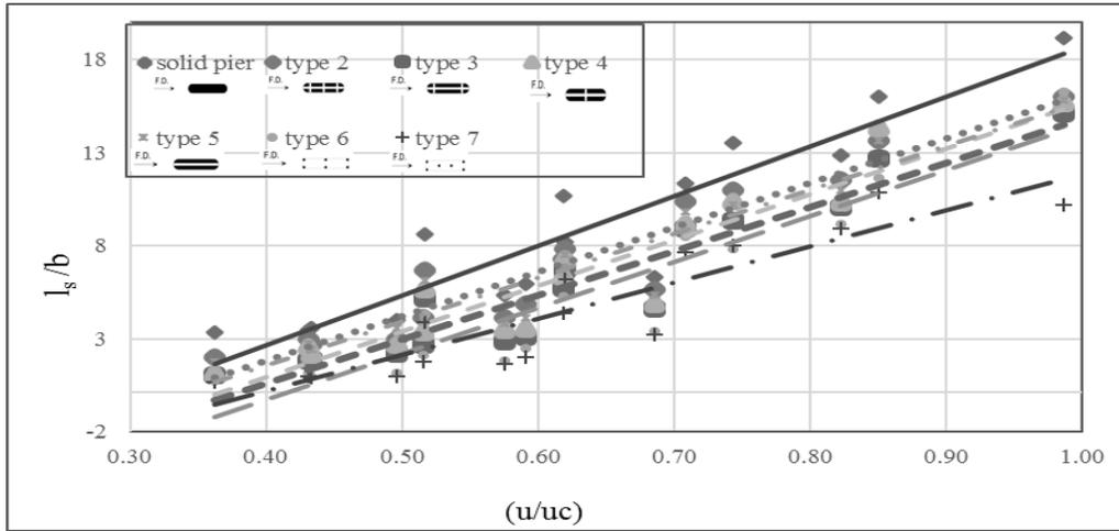
Fig.14. Values of relative scour depth ( $l_s/b$ ) versus  $(Q/b^2u)$  for different pier types.
