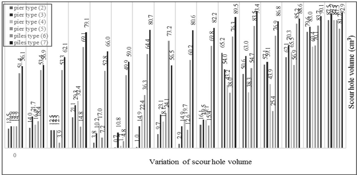
Fig.17. Values of scour hole volume (cm<sup>3</sup>) for different pier types at different discharges and upstream water levels.
