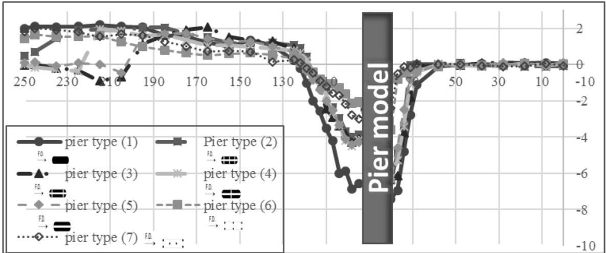
**Fig.6.** Longitudinal scour hole profile for studied pier types at  $Q = 18$  lit /s,  $y = 18.0$  cm and  $F_r = 0.25$ .
