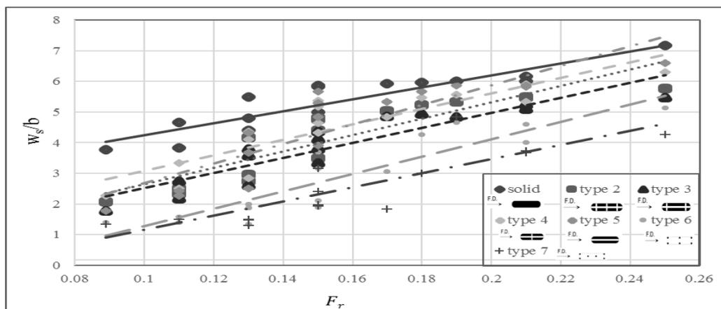
Fig.9. Values of relative scour hole width ( $w_s/b$ ) versus Froude number ( $F_r$ ) for different pier types.
