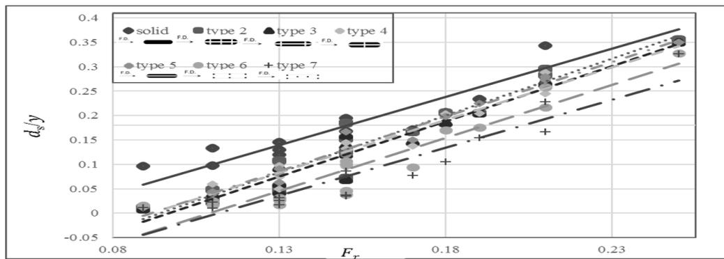
Fig.8. Values of relative scour hole depth ( $d_s/y$ ) versus Froude number ( $F_r$ ) for different pier types.
