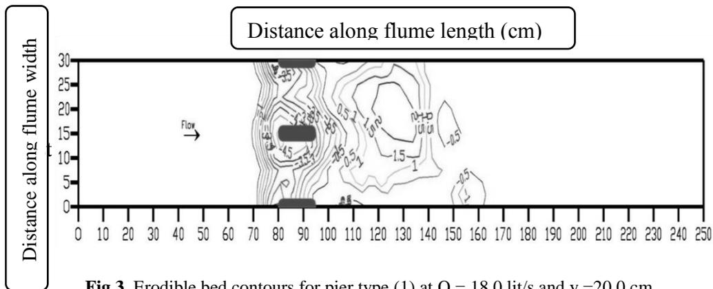
**Fig.3.** Erodible bed contours for pier type (1) at  $Q = 18.0$  lit/s and  $y = 20.0$  cm.
