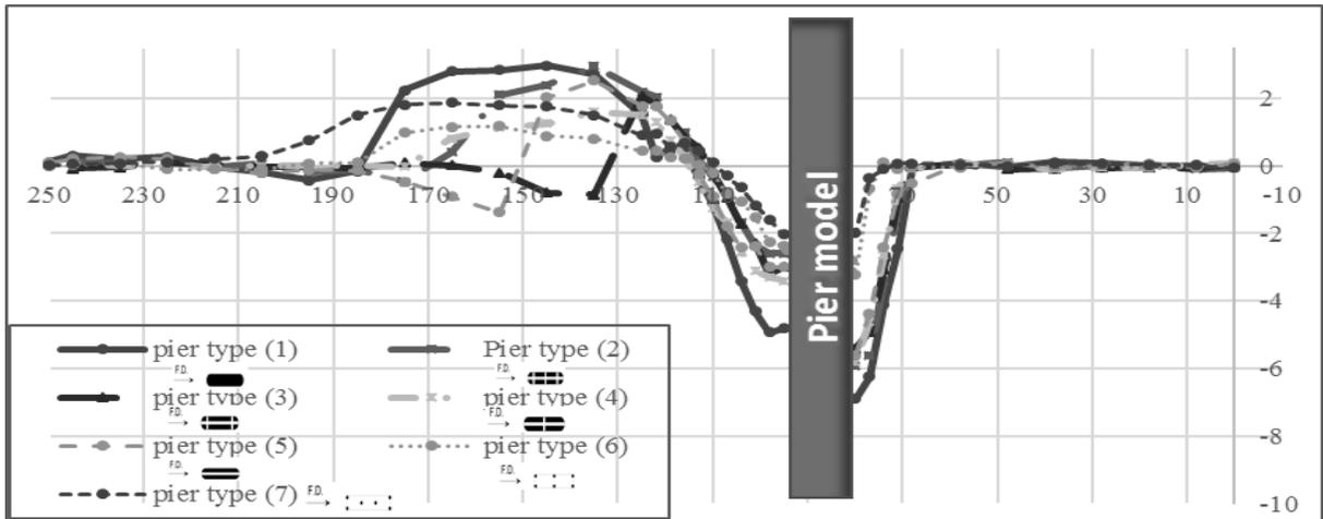
**Fig.7.** Longitudinal scour hole profile for studied pier types at  $Q = 18$  lit /s,  $y = 20.0$  cm and  $F_r = 0.21$ .
