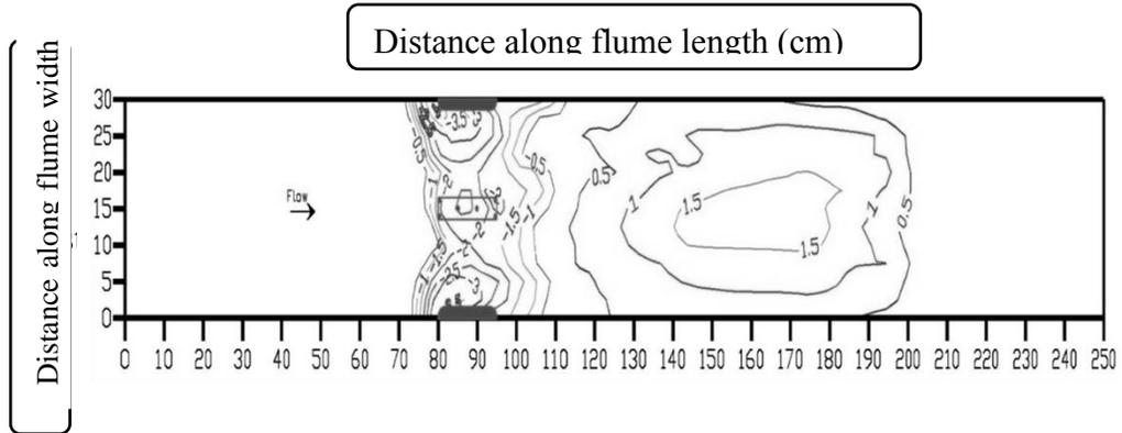
**Fig.5.** Erodible bed contours for pier type (7) at  $Q = 18.0$  lit/s and  $y = 20.0$  cm.
