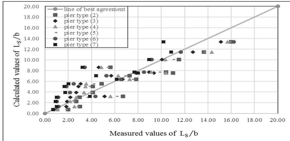
Fig. 20. Correlation between the regression model (Eq. 10) and the experimental data values for relative scour hole length ( $l_s/b$ ) for all pier types.
