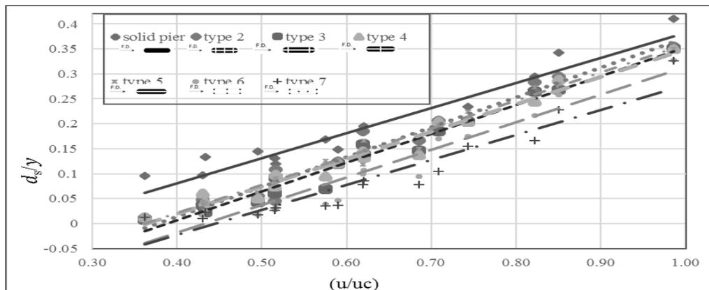
**Fig.11.** Values of relative scour hole depth ( $d_s/y$ ) versus ( $u/u_c$ ) for different pier types.
