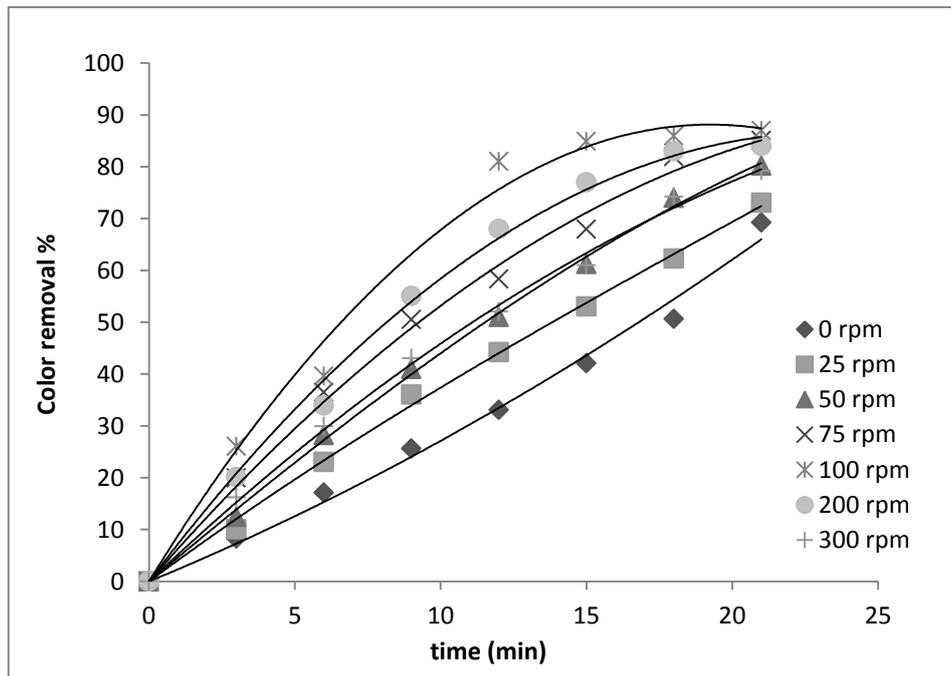
**Fig.2,** Color removal percentage vs. time at different agitation rotational speed, using screen cathode [C.D= 200 A/m<sup>2</sup>, C<sub>NaCl</sub> = 5 g/l, C<sub>0</sub> = 50 ppm]
