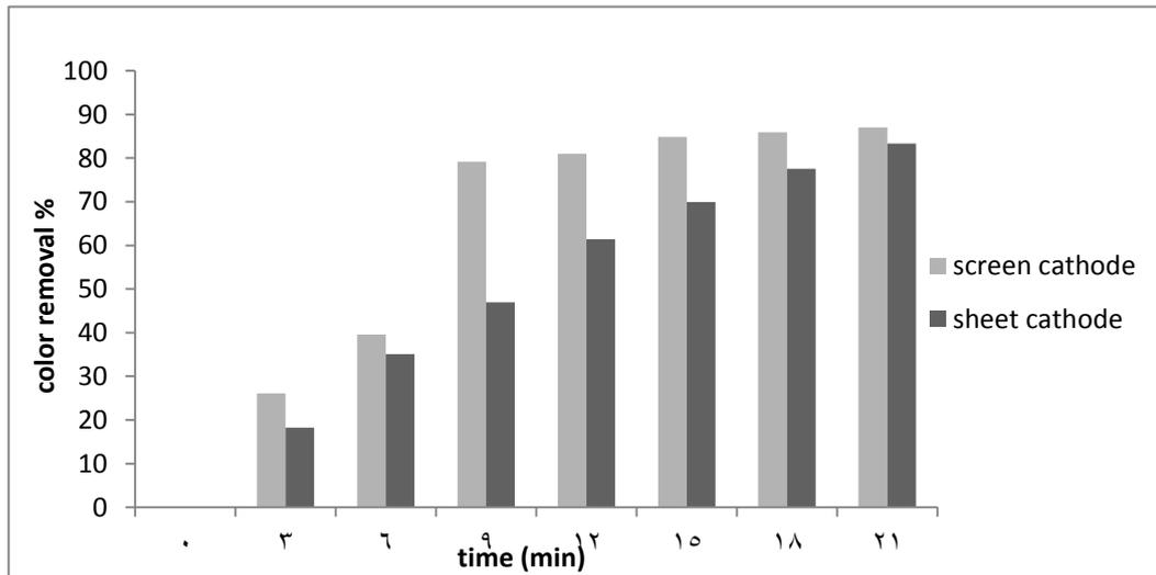
**Fig. 6:** Color removal percentage vs. time (min) using screen and vertical cylindrical sheet cathodes respectively [C.D= 200 A/m<sup>2</sup>, rotational speed =100 rpm, C<sub>NaCl</sub> = 5 g/l, C<sub>0</sub>= 50 ppm]
