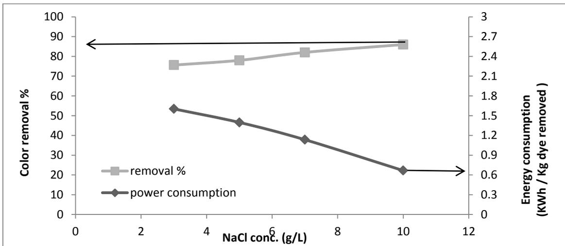
Fig. 4: Effect of initial NaCl concentration on the color removal efficiency and energy consumption, using screen cathode, [C<sub>0</sub> = 250 ppm, C.D= 125 A/m<sup>2</sup>, rotational speed = 100 rpm, time = 21 min]
