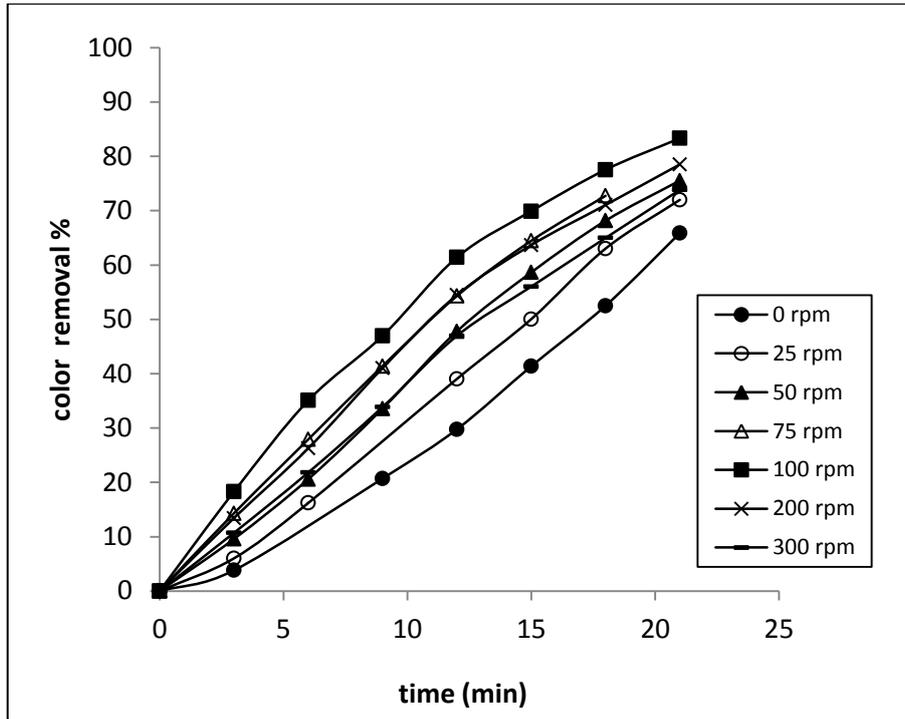
Fig.3: Color removal percentage vs. time at different rotational speed using sheet cathode [C.D= 200 A/m<sup>2</sup>, C<sub>NaCl</sub> = 5 g/l, C<sub>0</sub> = 50 ppm]
