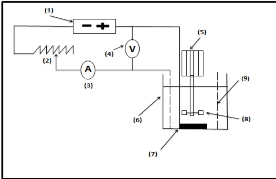
**Fig. 1:** Experimental set up of Batch EC reactor with screen cathode
