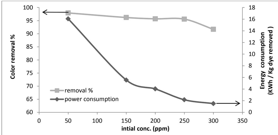
**Fig. 5:** Effect of initial conc. on the color removal efficiency and energy consumption, using vertical cylindrical screen cathode [C.D= 250 A/m<sup>2</sup>, rotational speed =100 rpm, C<sub>NaCl</sub> = 10 g/l, time = 21 min]
