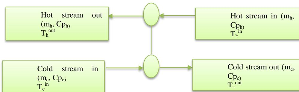
**Fig.2.** Variables required for the heat exchanger match.
