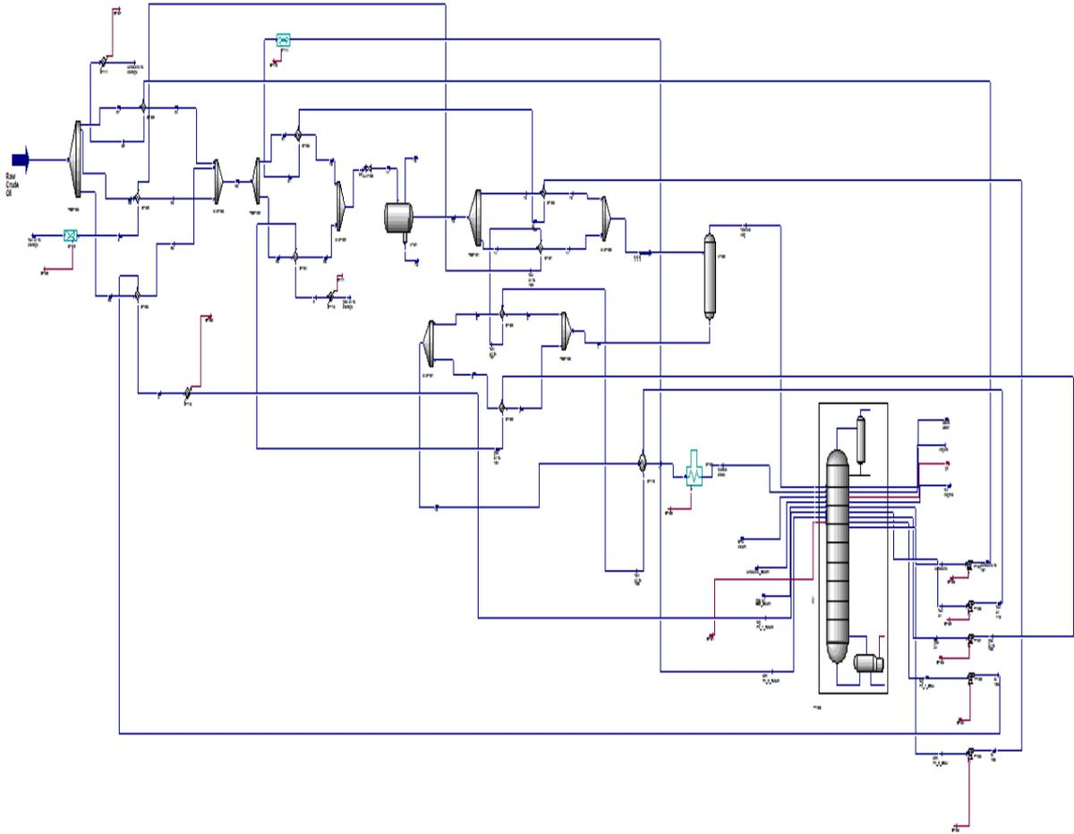
Fig.3. Case study simulation of Middle East CDU.
