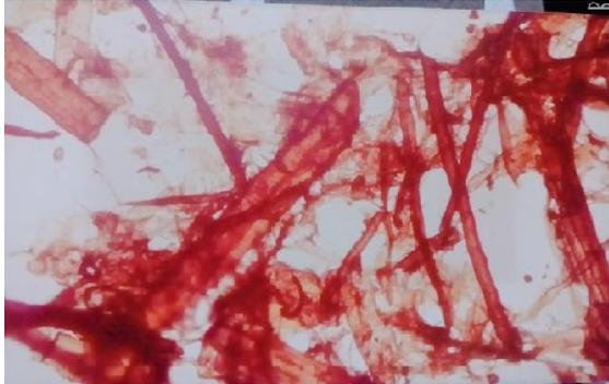
Fig.2. Mixture of all materials (fiber, vessel and pith) (40 X)
