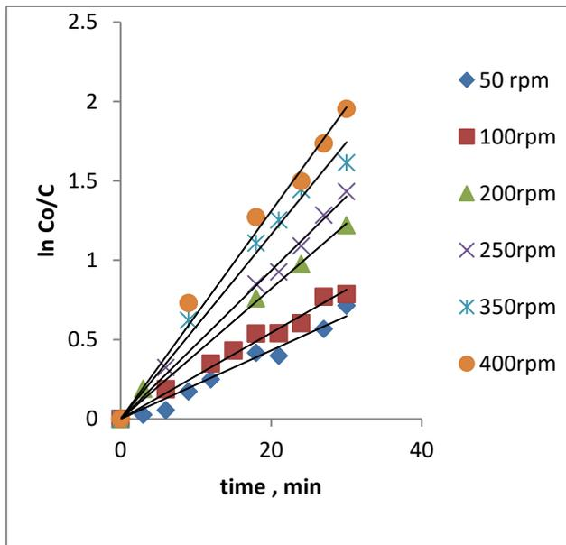
Fig.5. ln Co/C vs. time for 0.4% fiber- pulp consistency at different rpm.
