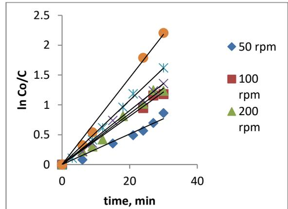
Fig.6. lnCo/C vs. time for 0.4% fine- pulp consistency at different rpm
