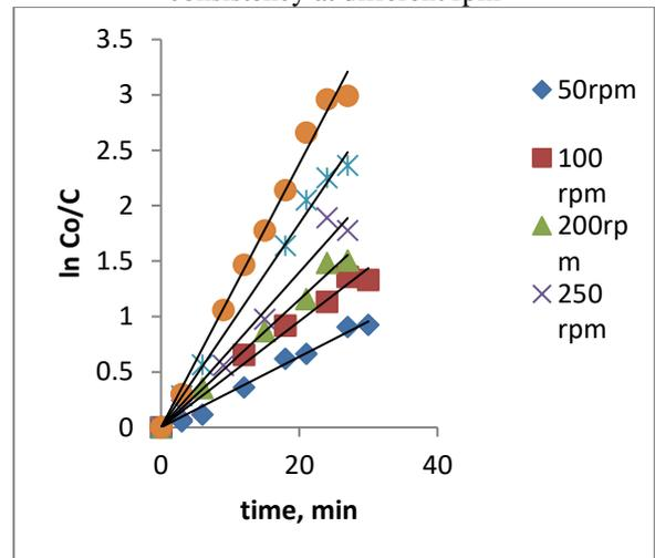
Fig.7. lnCo/C vs. time for 0.4% whole-pulp consistency at different rpm
