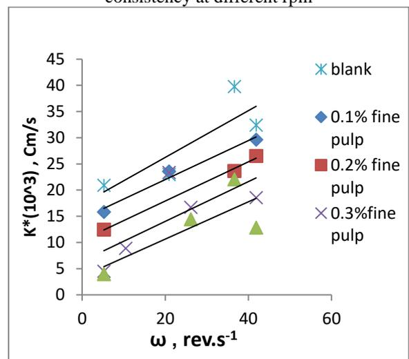
Fig.8. effect of impeller rotational speed on mass transfer coefficient at different whole- pulp consistency
