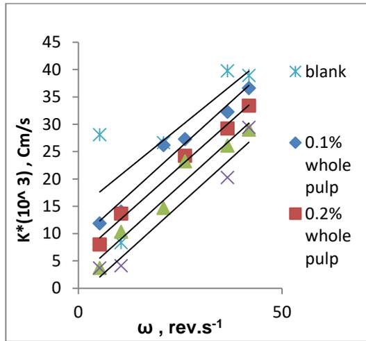
Fig.9. effect of impeller rotational speed on mass transfer coefficient at different fine- pulp consistency
