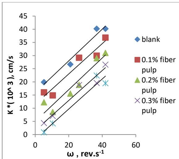
Fig.10. effect of impeller rotational speed on mass transfer coefficient at different fiber- pulp consistency
