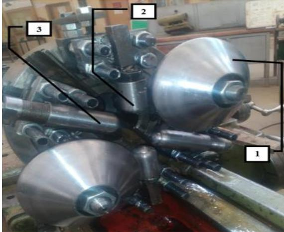
**Fig.1.** The completely new combined tool. (1) The rollers for conventional spinning (2) The balls for shear spinning (3) The balls for burnishing processes.
