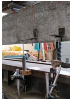
Figure 6: LVDTs location.
