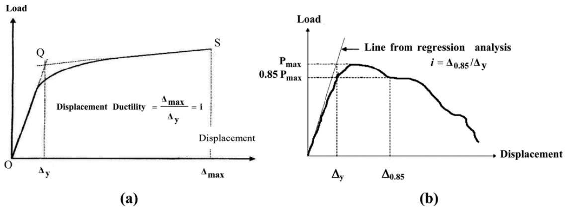
Figure 18 definition of displacement-ductility ratio.
