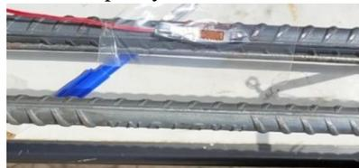
Figure 5: The used strain gauges.
