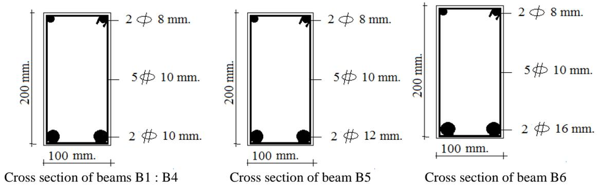
Figure 2: Cross section of the beam specimens
