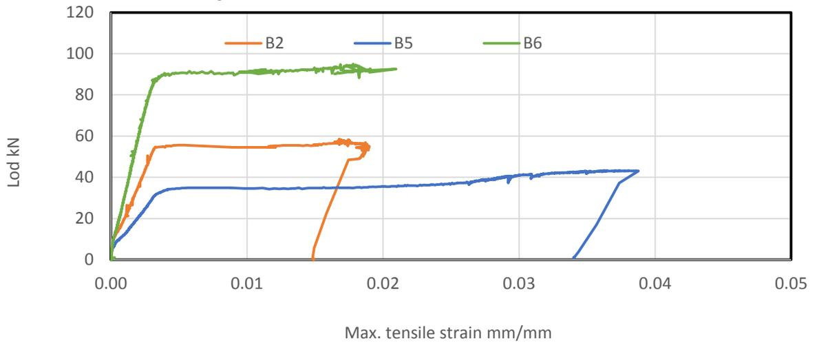
Figure 15: The relation between load and maximum tensile strain for beams B2, B5, and B6.
