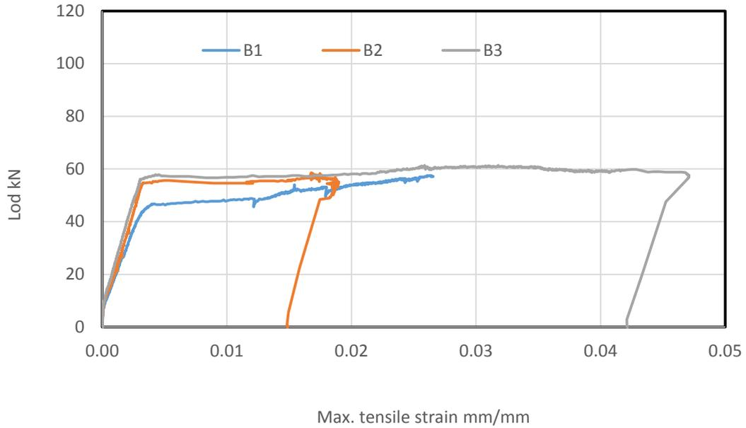
Figure 9: The relation between load and maximum tensile strain for beams B1: B3
