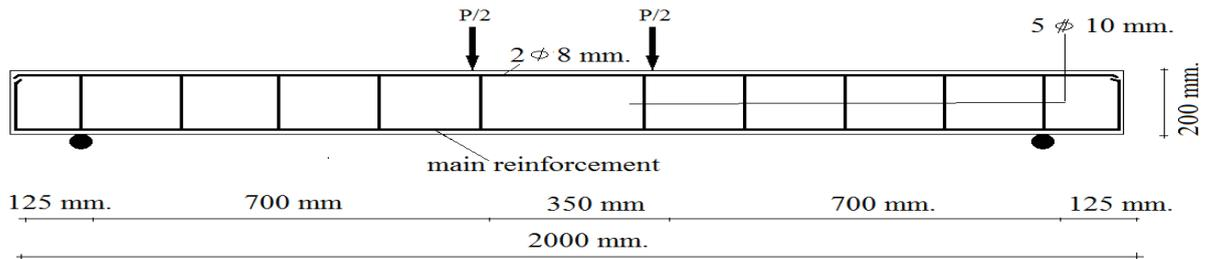
Figure 1: Beam dimensions, and reinforcement details.
