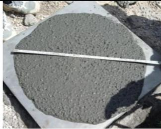
Figure 3: The slump flow test.
