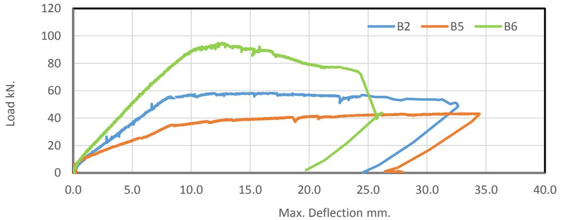
Figure 14: The relation between load and maximum deflection for beams B2, B5 and B6
