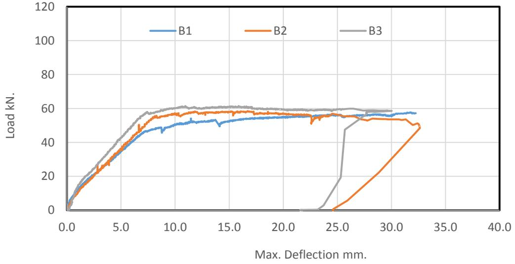
Figure 8: The relation between load and maximum deflection for beams B1: B3
