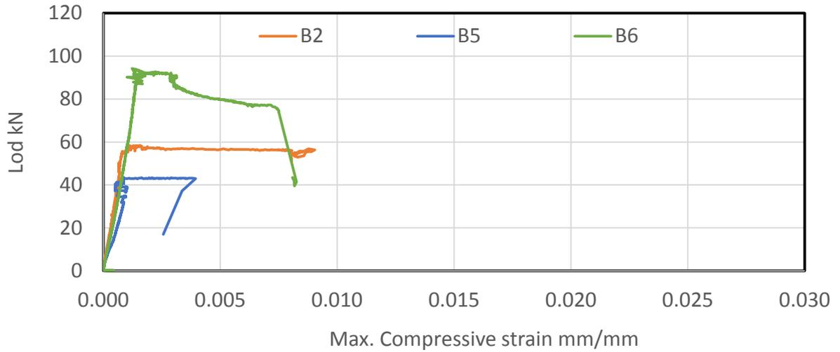
Figure 16: The relation between load and maximum compressive strain for beams B2, B5 and B6.
