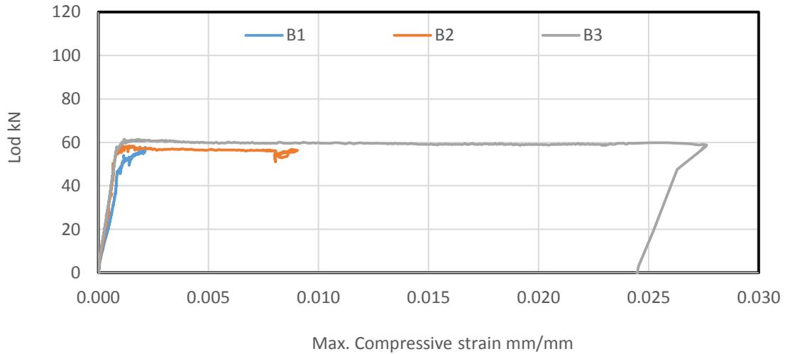
Figure 10: The relation between load and maximum compressive strain for beams B1: B3
