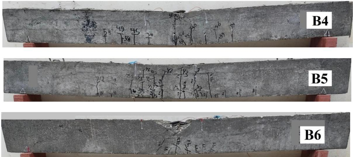
Figure 17: Cracking patterns and modes of failure at ultimate load for tested beams
