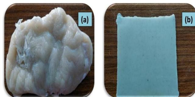
Figure 2. The shape of the prepared composites. (a) After melt mixing and (b) After compression.
