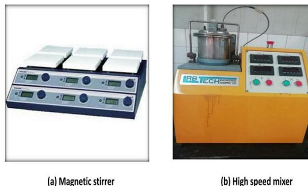
Figure 1. The Two instruments used in the clay modification (a) Magnetic stirrer and (b) High speed mixer.
