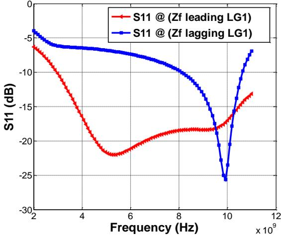
Figure 5. Simulated input return loss (S11) with respect to frequency for  $Z_{in}(= Z_g // Z_{F_{in}}; Z_F$  leading  $L_{G1}$ ) of the suggested topology in Figure 4 (B), and  $Z'_{in}$  ( $; Z_F$  lagging  $L_{G1}$ ) of the regular topology in Figure 4 (A)
