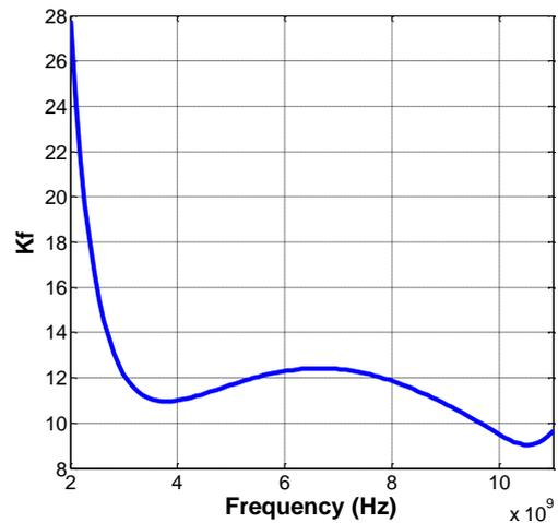
Figure 14. Simulation result of the stability factor (Kf)
