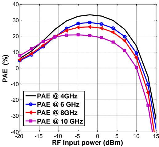
Figure 12. Simulation results of the power added efficiency (PAE)
