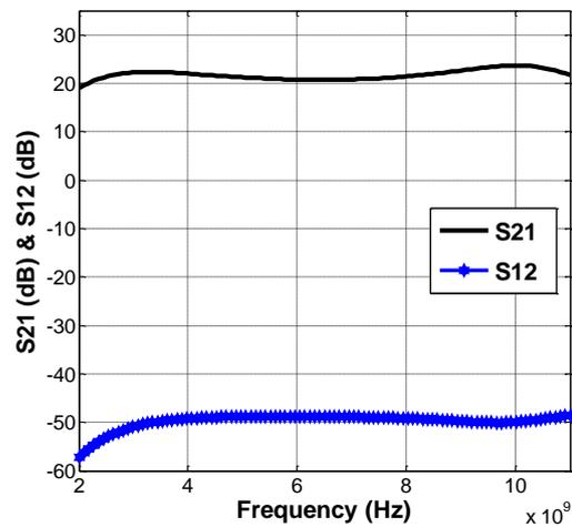
Figure 10. The simulation results of the power gain (S21) and the reverse isolation (S12)
