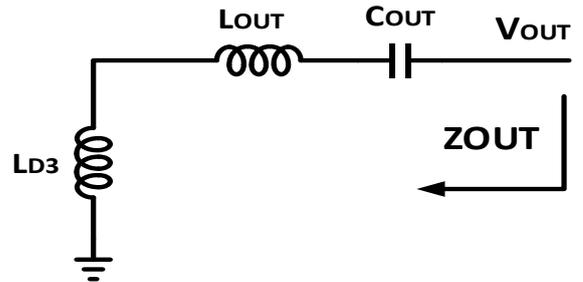
Figure 7. Small-signal equivalent circuit for the output impedance
