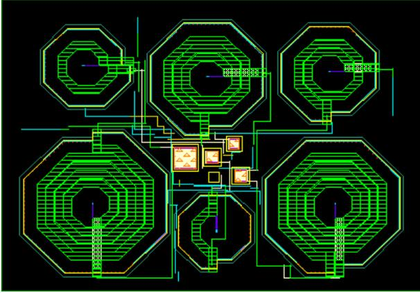
Figure 8. The layout of the recommended UWB PA
