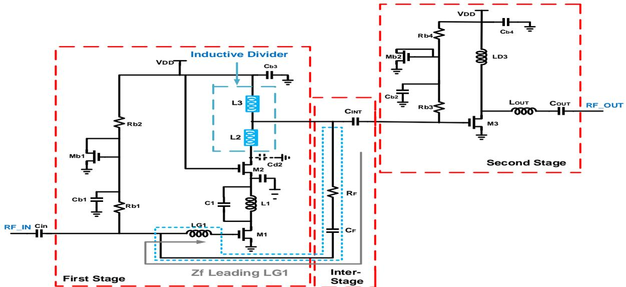
Figure 1. Complete schematic of the recommended UWB-power amplifier
