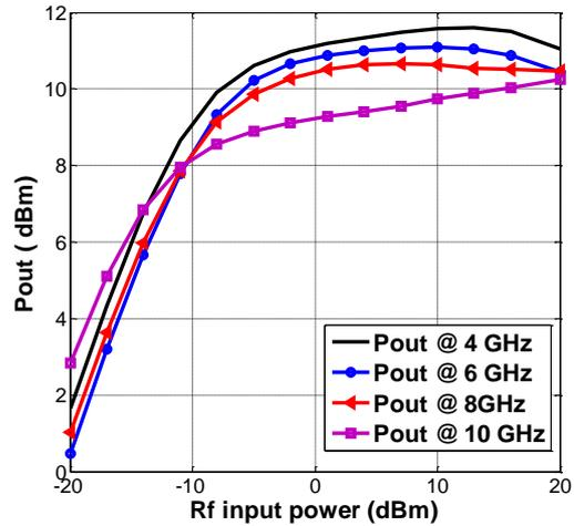
Figure 13. Simulation results of the output power ( $P_{out}$ )
