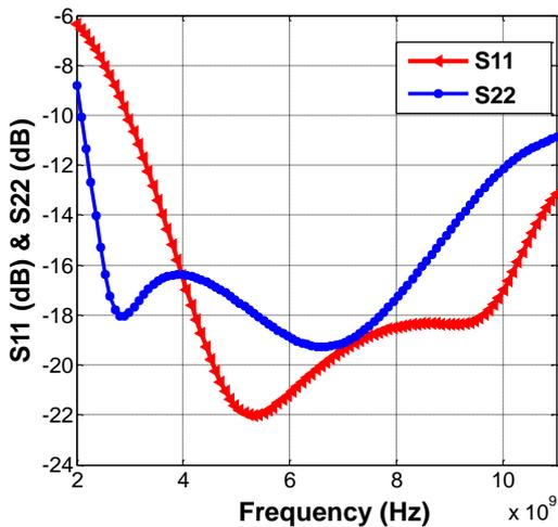
Figure 9. Simulation results of the input return loss (S11) and the output return loss (S22)
