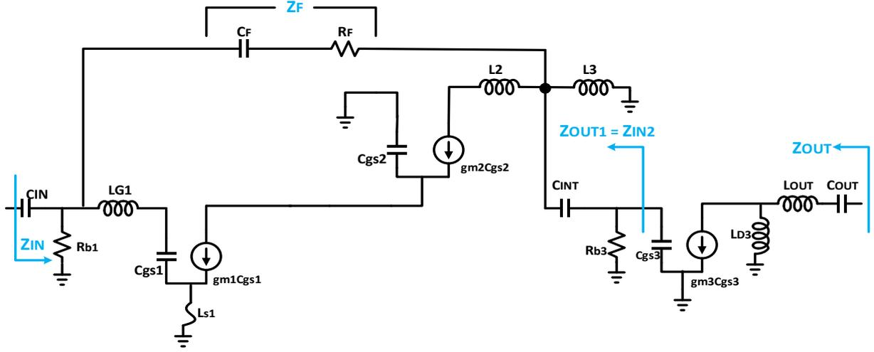
Figure 2. A small-signal equivalent circuit of the recommended UWB-power amplifier
