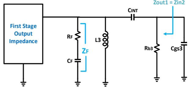
Figure 6. Small-signal equivalent circuit for the interstage matching
