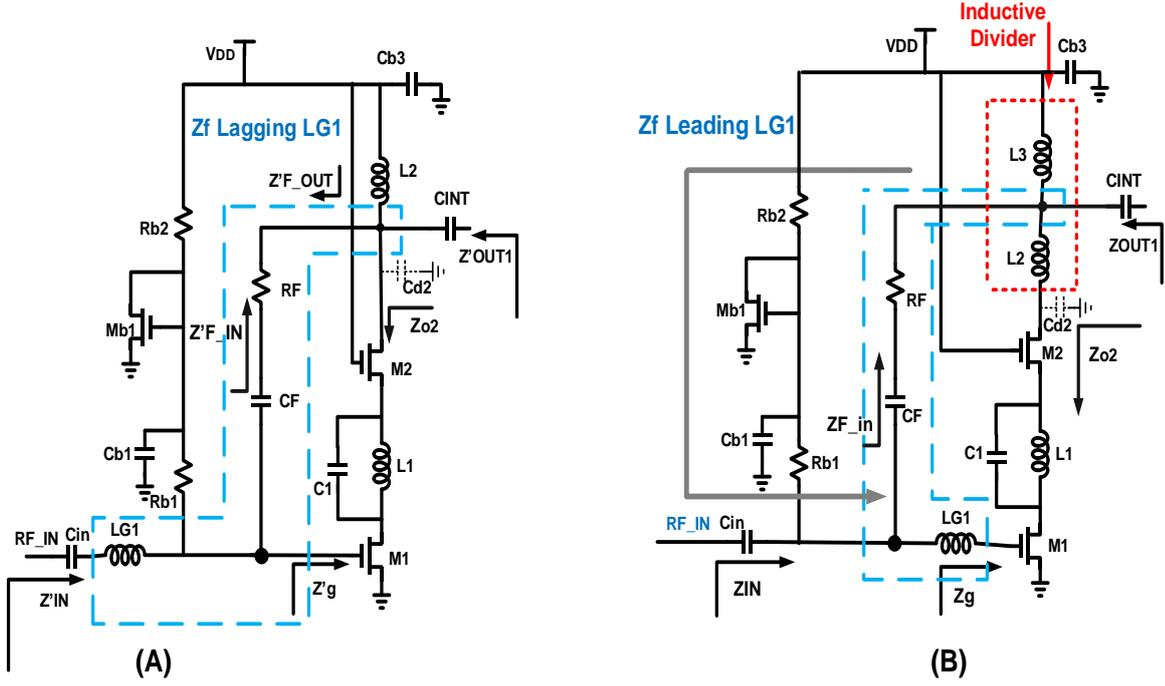
Figure 4. A circuit with wideband input matching topologies (A) a regular matching with feedback circuit ( $Z_F$  lagging the gate inductor  $L_{G1}$ ) without the inductive divider, and (B) a proposed wideband input matching topology (feedback circuit  $Z_F$  leading the gate inductor  $L_{G1}$ ) combining with the peaking inductor divider
