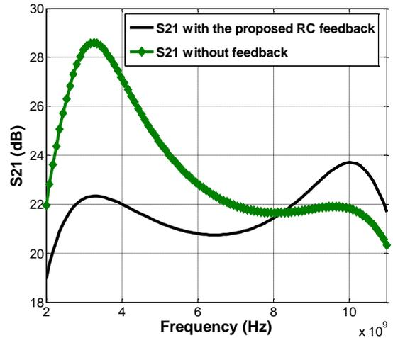
Figure 3. Influence of the shunt feedback ( $R_F$  and  $C_F$ ) on the gain flatness of the recommended UWB-PA
