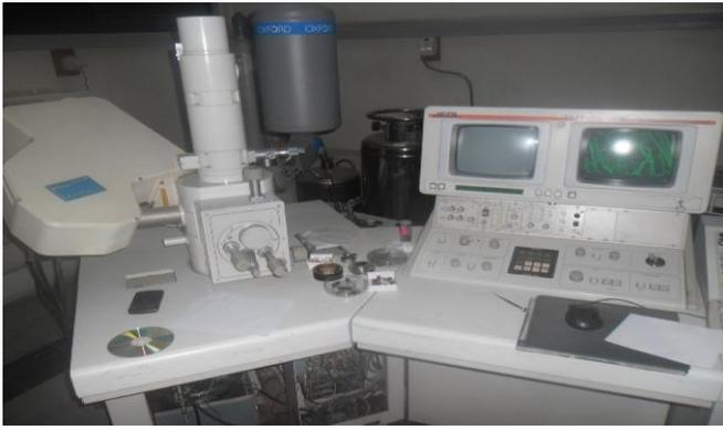
Figure 5: The scanning electron microscope (SEM) device
