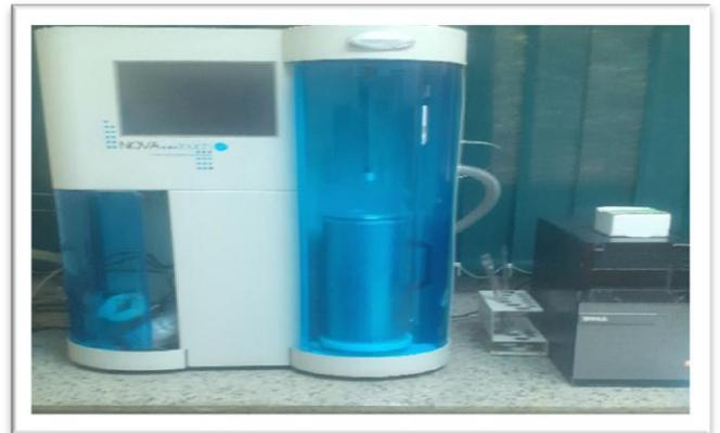
Figure 4: NOVA touch 4LX instrument
