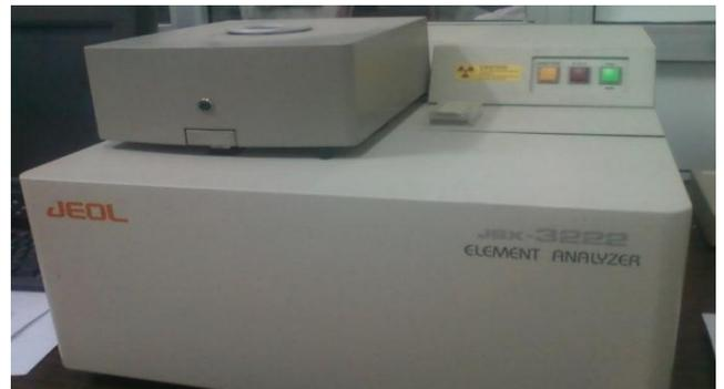
Figure 3: X-ray fluorescence analysis (XRF) test apparatus
