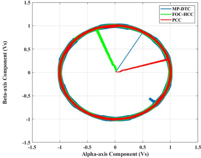
**Figure 36: The loci of the IM stator flux under both the FOC-HCC and the PCC technique**
