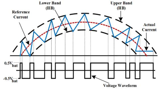
Figure 3: The hysteresis current controller concept
