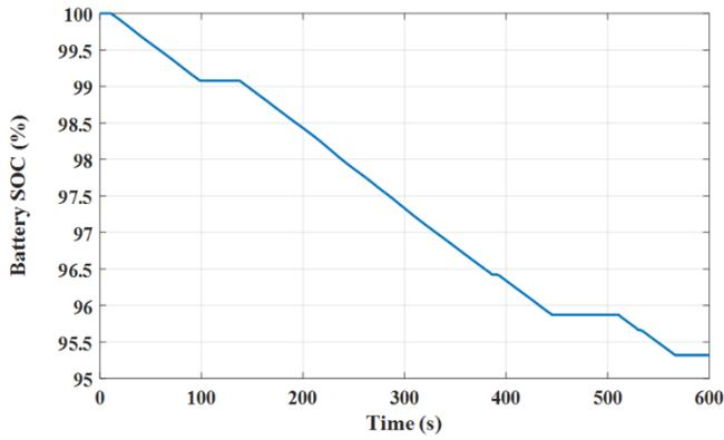
Figure 15: The EV battery state of charge under the FOC-HCC technique
