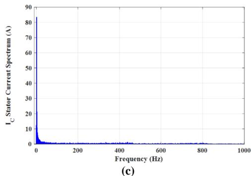
Figure 12: The IM stator currents spectrum under the FOC-HCC technique, (a) phase a current spectrum; (b) phase b current spectrum; (c) phase c current spectrum
