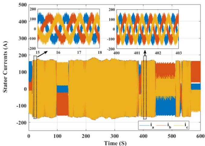
Figure 11: The IM stator currents under the FOC-HCC technique
