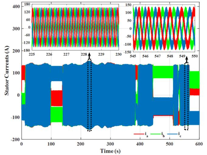
Figure 29: The three-phase stator currents under the PCC technique
