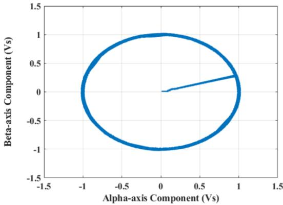
**Figure 31: The stator flux loci under the PCC technique**
