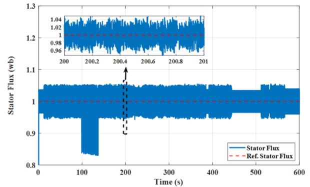
Figure 19: The IM stator flux under the MP-DTC technique
