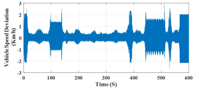
Figure 8: The deviation of EV speed from the WLTP reference under the FOC-HCC technique
