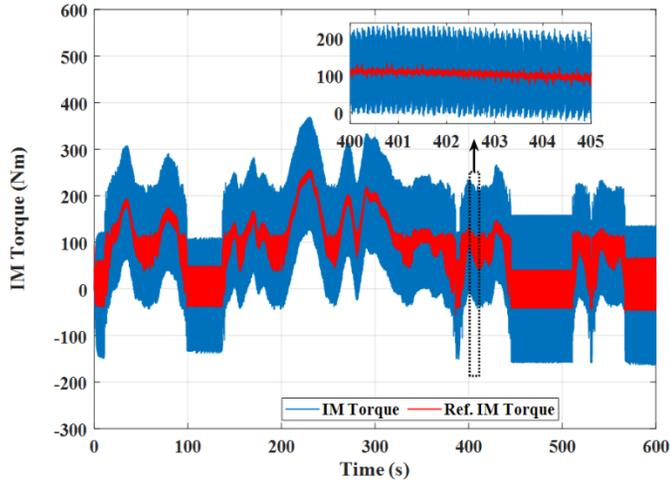
Figure 27: The IM developed torque under the PCC technique
