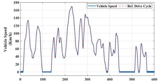
Figure 7: The EV speed based on the FOC-HCC technique
