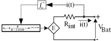
Figure 2: The EV battery equivalent circuit
