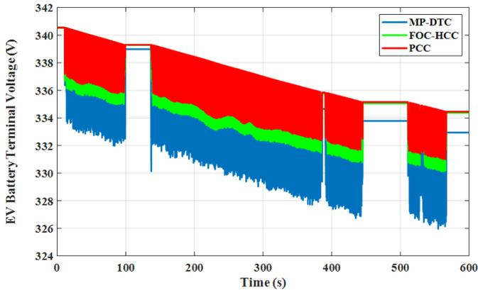
**Figure 37: The EV battery terminal voltage under both the FOC-HCC and the PCC technique**
