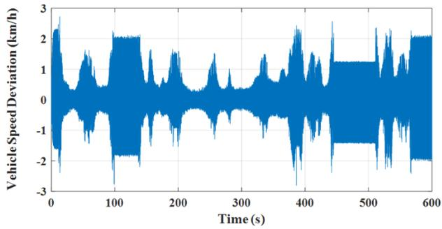
Figure 26: The deviation of EV speed from the WLTP reference under the PCC technique
