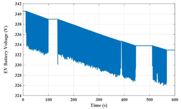
Figure 23: The EV battery terminal voltage under the MP-DTC technique
