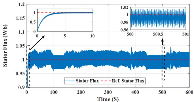
Figure 10: The IM stator flux under the FOC-HCC technique
