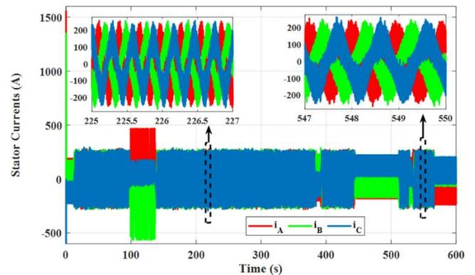
Figure 20: The IM stator currents under the MP-DTC technique
