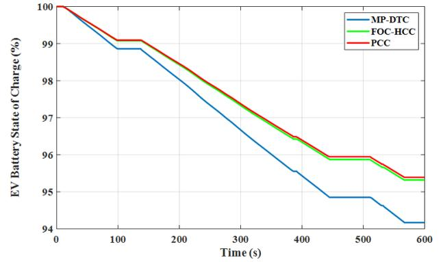
**Figure 38: The EV battery state of charge under both the FOC-HCC and the PCC technique**
