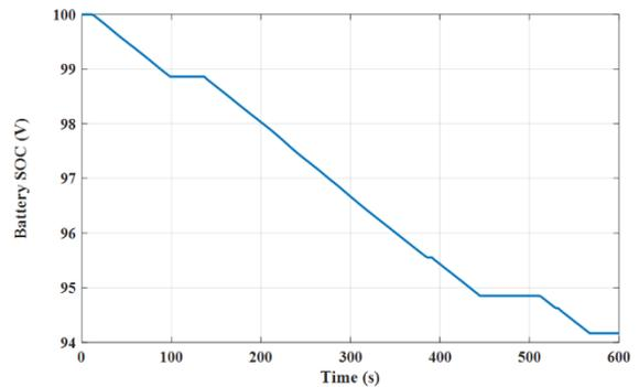
Figure 24: The EV battery state of charge under the MP-DTC technique
