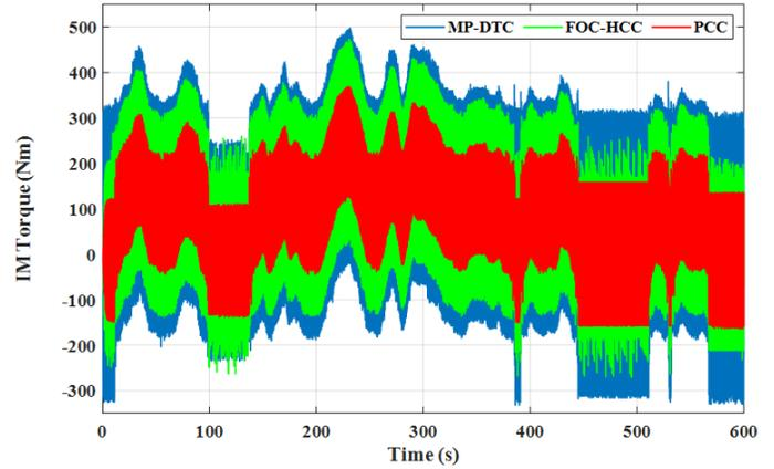
**Figure 34: The IM developed torque under both the FOC-HCC and the PCC technique**
