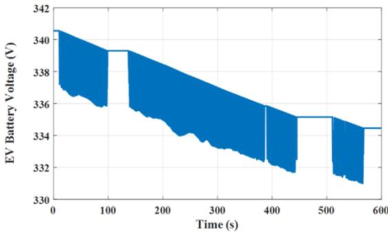
**Figure 32: The terminal voltage across the EV battery under the PCC technique**
