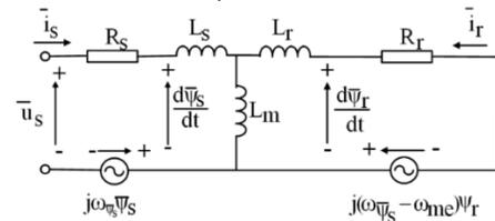
Figure 1: The IM per phase equivalent circuit
