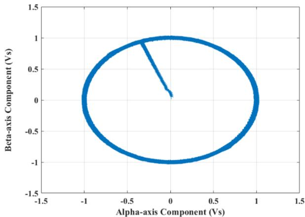
Figure 13: The IM stator flux loci under the FOC-HCC technique
