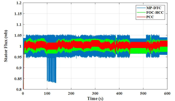
**Figure 35: The IM stator flux under both the FOC-HCC and the PCC technique**
