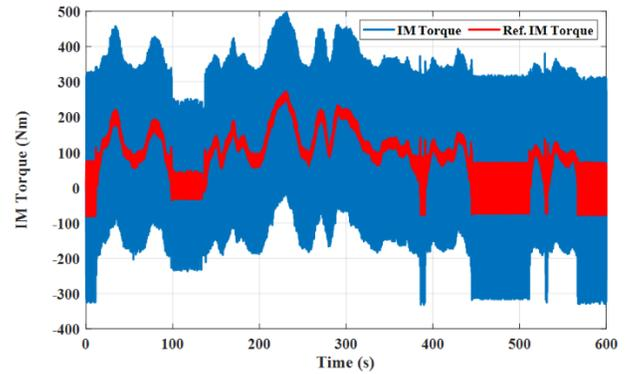
Figure 18: The IM torque under the MP-DTC technique
