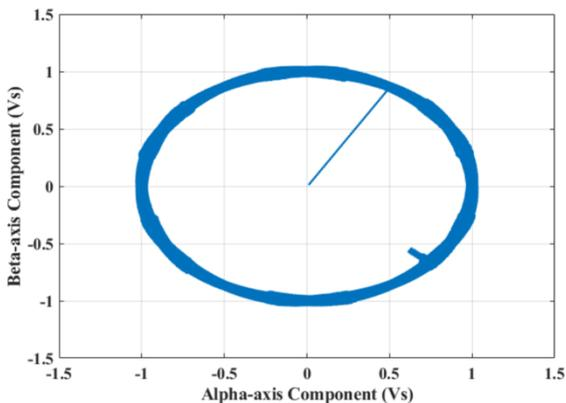
Figure 22: The stator flux loci under the MP-DTC technique
