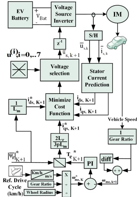
Figure 6: Block diagram of the PCC for IM in an EV system
