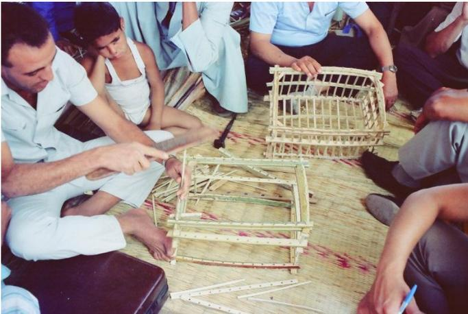
Figure 5 The making of a traditional date palm midribs crate.
