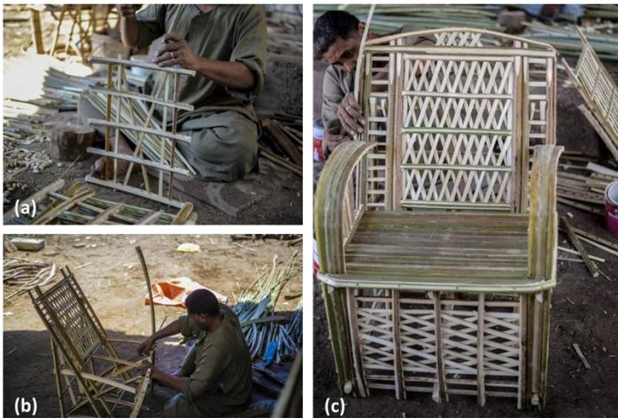
Figure 6 Prefabrication of a traditional date palm midrib chair. (a) Creating a lattice for the back of the chair. (b) The structure of the chair. (c) A completed chair.
