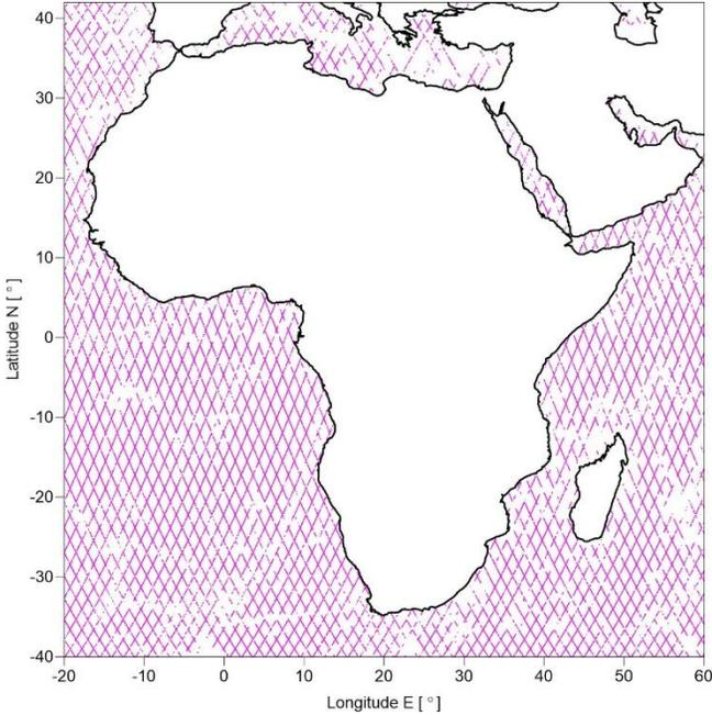
Figure 3. Locations of the altimetry-derived gravity data for Africa.
