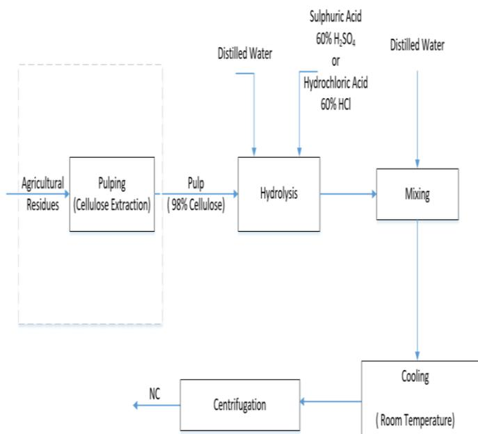
**Figure 1: NC manufacturing block flow diagram from pulp**
