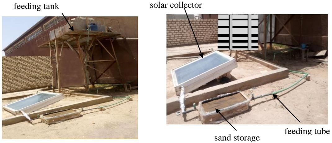
Figure 2 Photos for the Experimental Set-up with Different Components.
