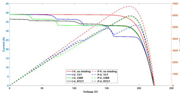
Figure 12. (I-V) and (P-V) characteristic curves of the PV system under shading pattern No. 4
