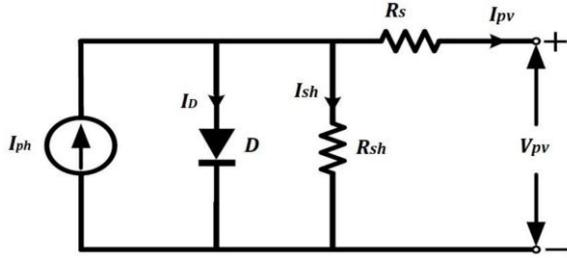
Figure 1. Single diode model
