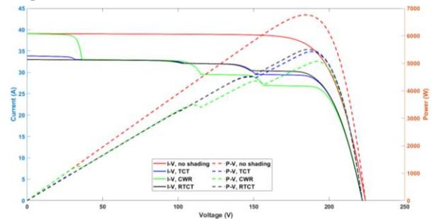
Figure 13. (I-V) and (P-V) characteristic curves of the PV system under shading pattern No. 5
