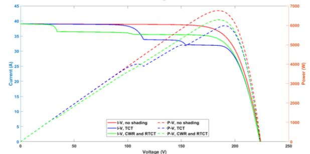
Figure 10. (I-V) and (P-V) characteristic curves of the PV system under shading pattern No. 2
