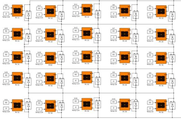
Figure 15. The 5x5 system showing the bypassing diodes
