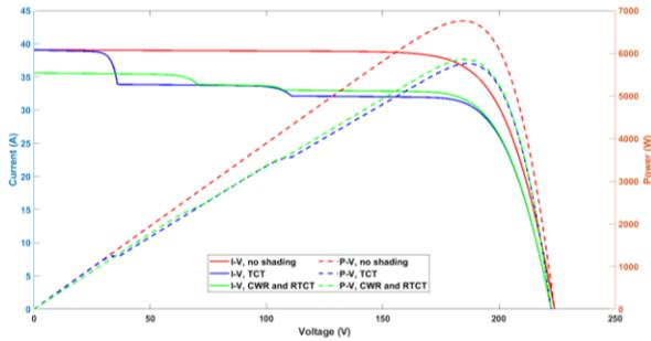
Figure 11. (I-V) and (P-V) characteristic curves of the PV system under shading pattern No. 3
