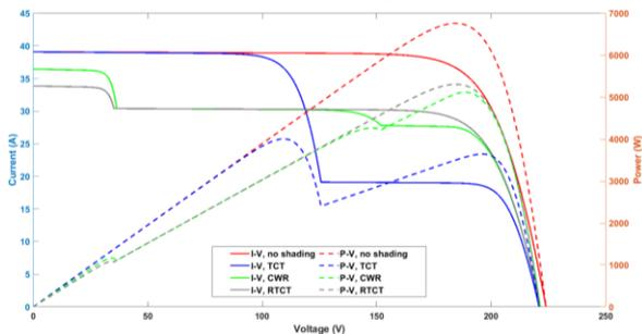
Figure 9. (I-V) and (P-V) characteristic curves of the PV system under shading pattern No. 1
