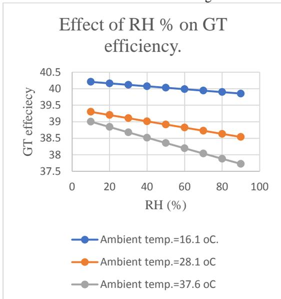
Fig.24 The effect of air relative humidity ratio on GT efficiency.
