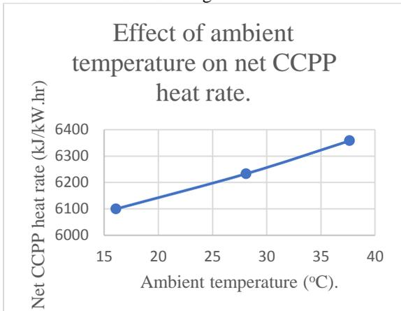
Fig. 16 The effect of ambient temperature on combined cycle power plant (CCPP) net heat rate.
