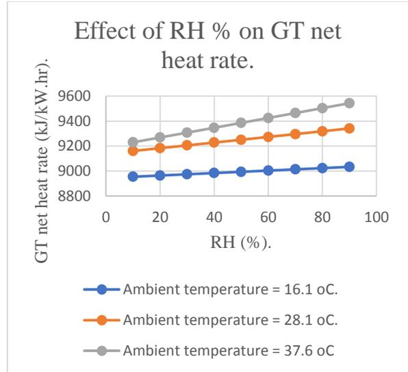
Fig. 25 the effect of air relative humidity ratio (RH) on gas turbine (GT) net heat rate.
