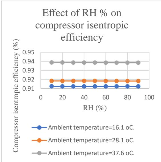
Fig. 19 The effect of air relative humidity ratio on compressor isotropic efficiency.
