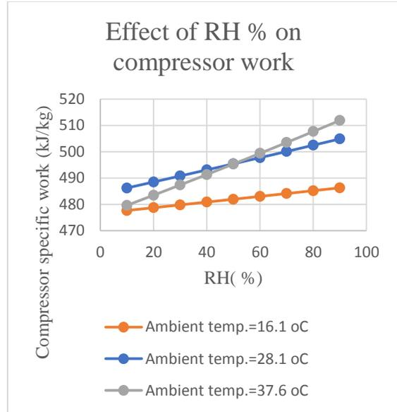
Fig. 17 The effect of air relative humidity on compressor specific work.
