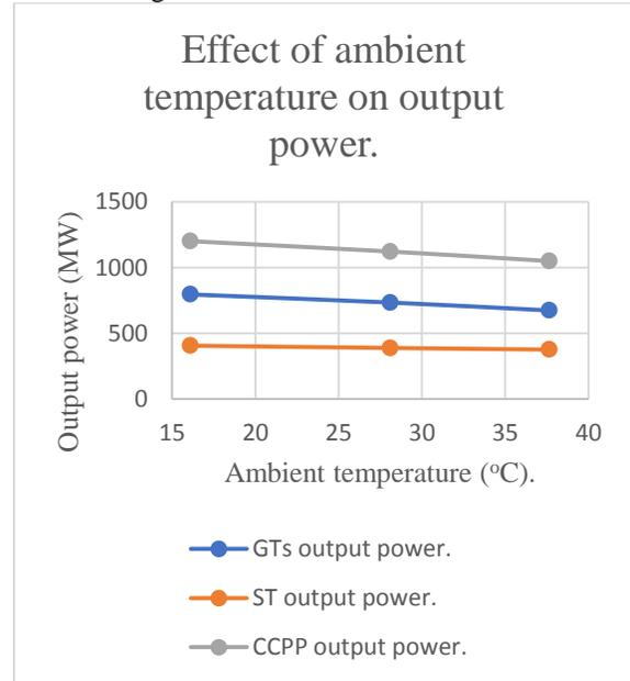
Fig. 14 The effect of ambient temperature on output gross power.
