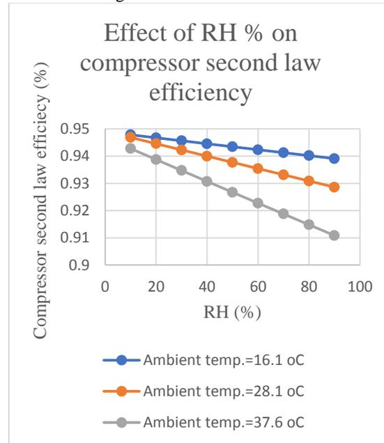
Fig.22 The effect of air relative humidity ratio on compressor second law efficiency.
