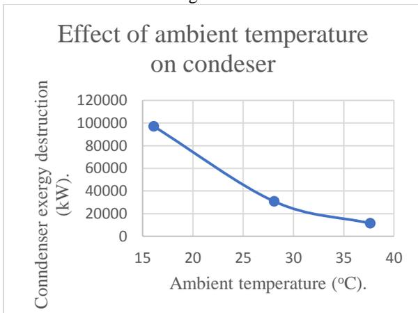
Fig. 12 The effect of ambient temperature on condenser exergy destruction.
