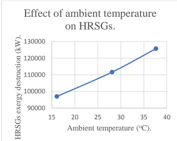
Fig.7 The effect of ambient temperature on heat recovery steam generators (HRSGs) exergy destruction.
