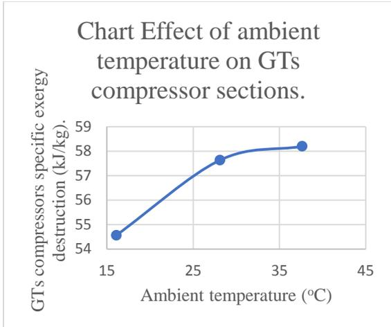
Fig. 3 The effect of ambient temperature on compressor exergy destruction.
