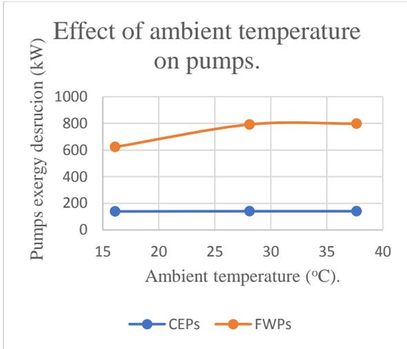
Fig. 11 The effect of ambient temperature on pumps exergy destruction.
