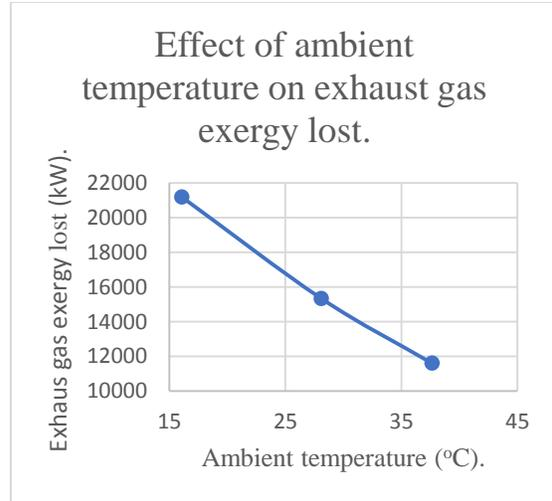
Fig. 9 The effect of ambient temperature on exhaust gases exergy lost.
