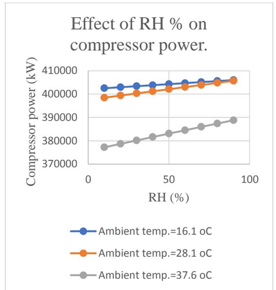
Fig.18 The effect of air relative humidity on compressor power.
