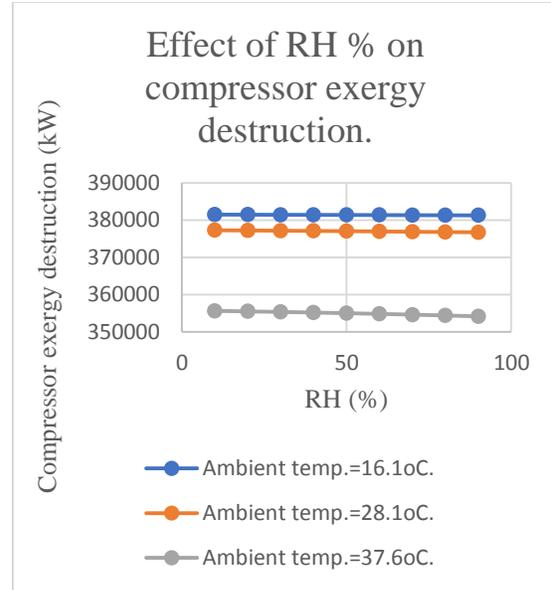
Fig.21 The effect of air relative humidity ratio on compressor exergy destruction rate.
