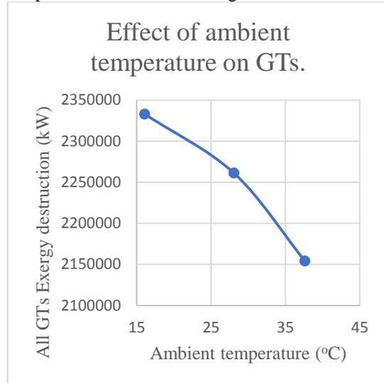
Fig. 6 The effect of ambient temperature on overall gas turbine (GT) exergy destruction.
