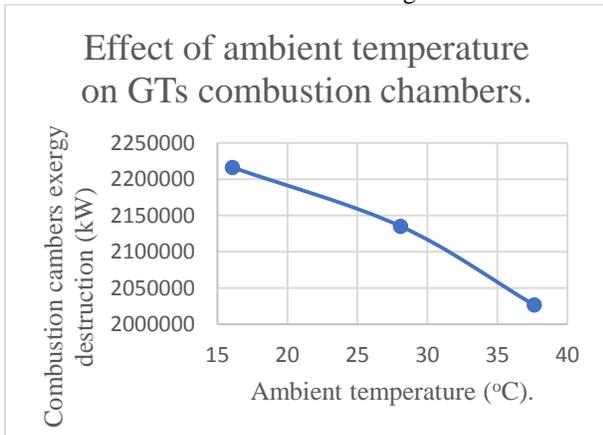
Fig. 4 The effect of ambient temperature on GT combustion chambers exergy destructions.
