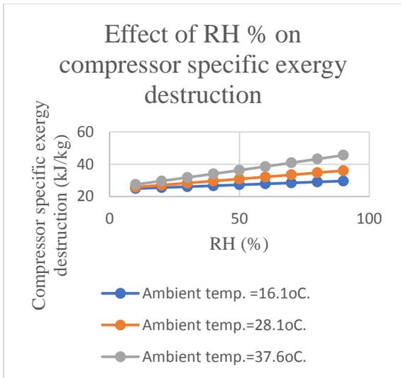
Fig. 20 The effect of air relative humidity on compressor specific exergy destruction
