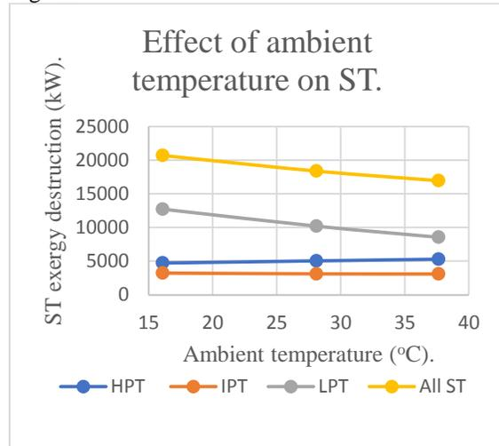
Fig. 10 The effect of ambient temperature on steam turbine (ST) exergy destruction.
