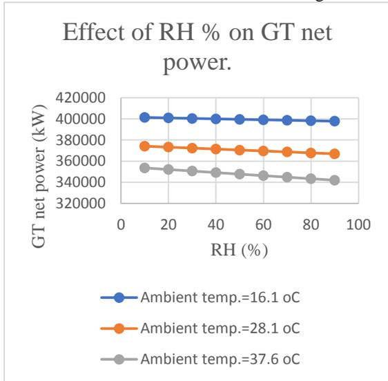
Fig. 23 effect of air relative humidity ratio on GT net power.
