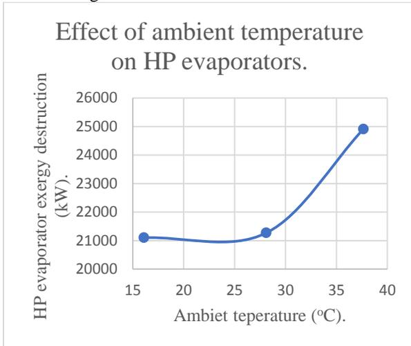
Fig. 8 The effect of ambient temperature on HP evaporator exergy destruction.
