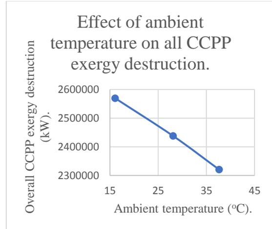
Fig. 13 The effect of ambient temperature on overall combined cycle power plant (CCPP) exergy destruction.
