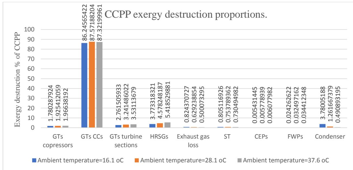
Fig. 2 The proportions of the combined cycle power plant (CCPP) components exergy destruction.
