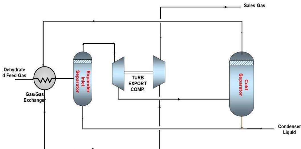
Figure 3: PFD for a Typical Turbo-Expansion Unit [13]
