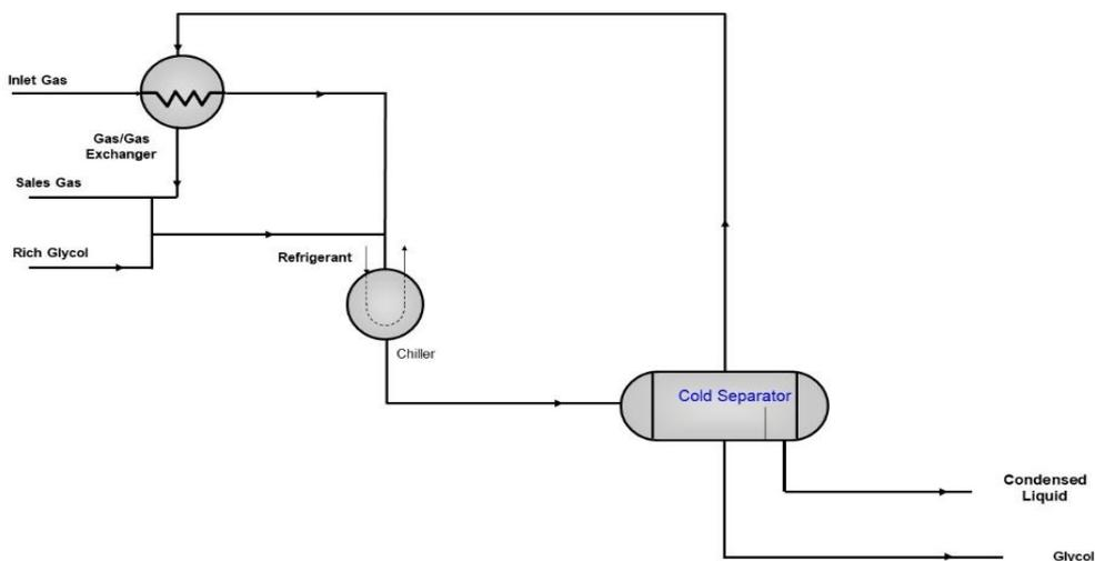
Figure 2: PFD for a Basic Mechanical Refrigeration unit [10]
