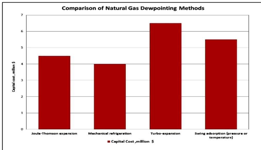
**Figure 8: Capital Cost for different natural gas hydrocarbon dew pointing control methods**
