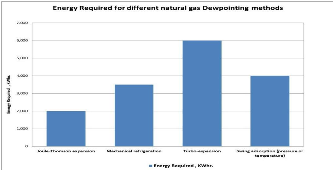
**Figure 7: Energy Required for different Natural Gas Hydrocarbon Dewpointing Control Methods**
