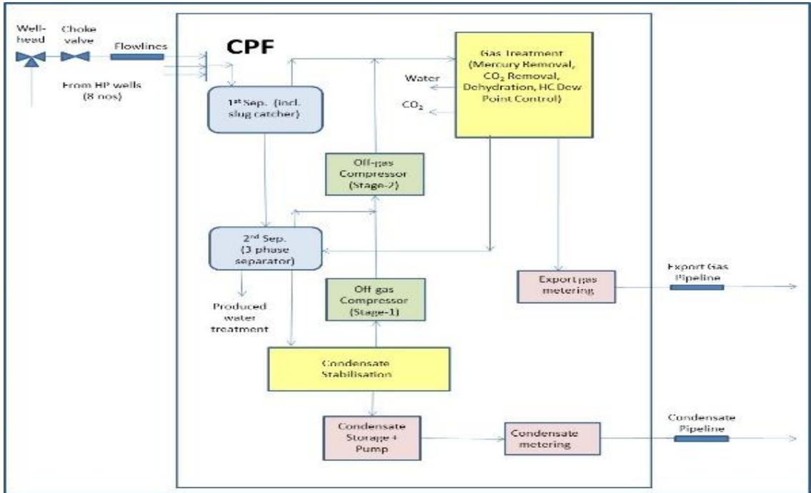
Figure 1 Schematic of the CPF Process Units
