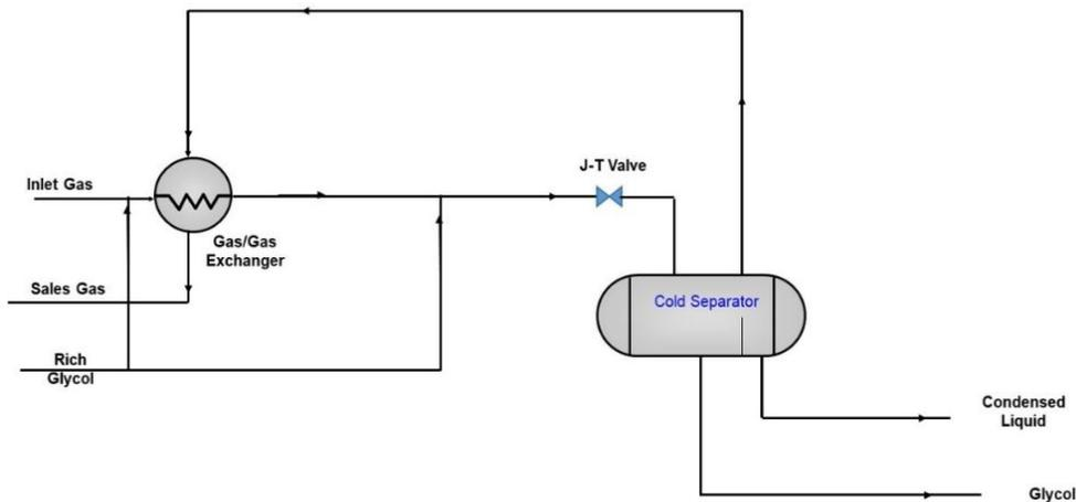
Figure 1: PFD for a typical Joule-Thomson Expansion unit [7]
