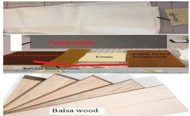
Fig.1 Raw materials of cores and skins
