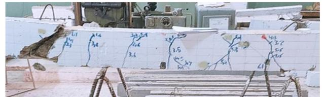
Picture.4. Mode of failure of beam (D1).
