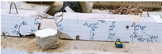
Picture.7. Mode of failure of beam (D4).
