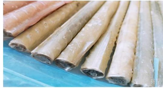
Picture.1. Cross-section view of the FRP Hybrid Bar.
