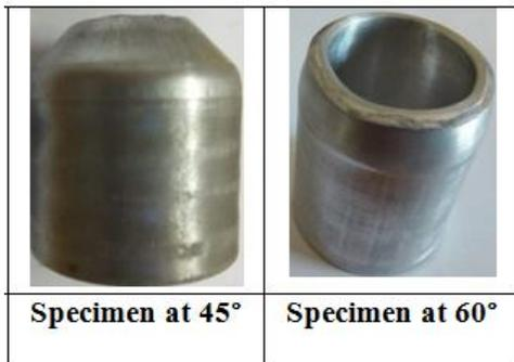
Fig.11 the deformed tubes after nosing process.
