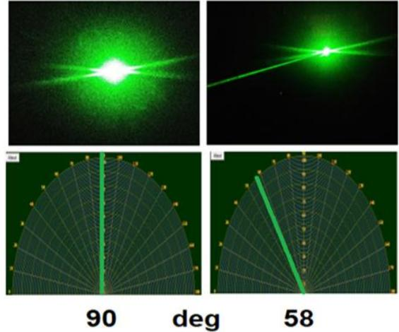
Figure.12. the real images were captured by proposed system and identify the angle of laser beam ( $90^\circ$ ) on axis And ( $58^\circ$ ) off axis
