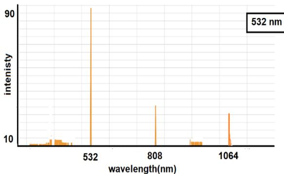
Figure.11. the spectrum after passing through the diffraction grating and then recorded by the sky camera for laser emitted at wavelength  $\lambda = 532$  nm
