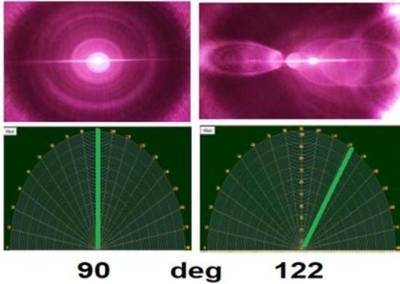
Figure.15. The real images were captured by the proposed system and identify the angle of laser beam (90°) on axis and (122°) off axis
