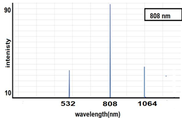
Figure.14. the spectrum after passing through the diffraction grating and then recorded by the sky camera for laser emitted at wavelength  $\lambda = 808$  nm
