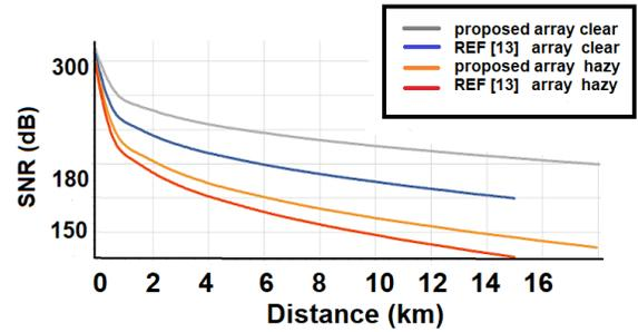
Figure.5. SNR for the proposed optical array in clear and hazy atmospheric conditions compared to the work in [13]
