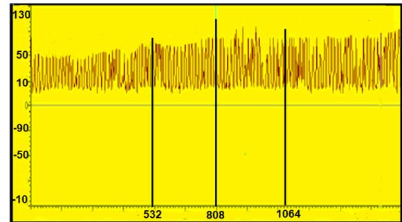
Figure13.808 nm laser real measurement formed by spectrometer before using proposed system
