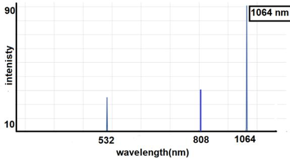
Figure 16.The spectrum after passing through The diffraction grating and then recorded by the sky
