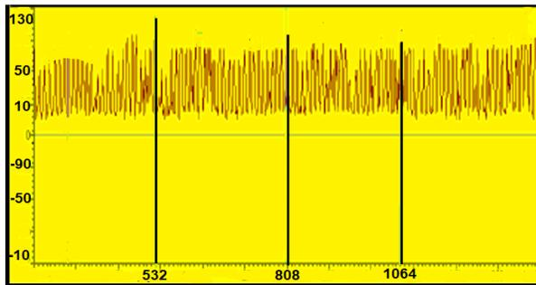
Figure.10.532 nm laser real measurement formed by Spectrometer before using proposed system.
