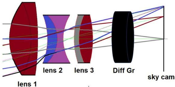
Figure.2. 2-D schematic of the proposed optical
