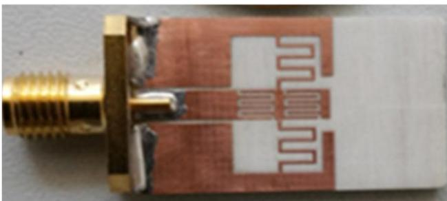
Fig. 7. A photo of the fabricated CRLH-antenna prototype.
