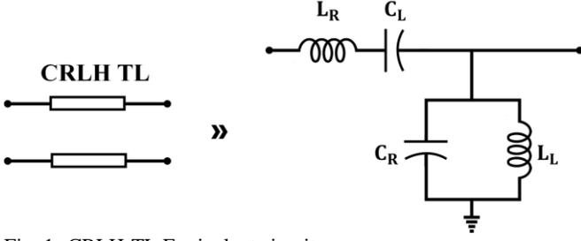
Fig. 1. CRLH-TL Equivalent circuit.
