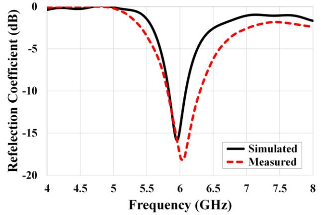
Fig. 8. The measured and simulation reflection coefficient of the CRLH antenna.
