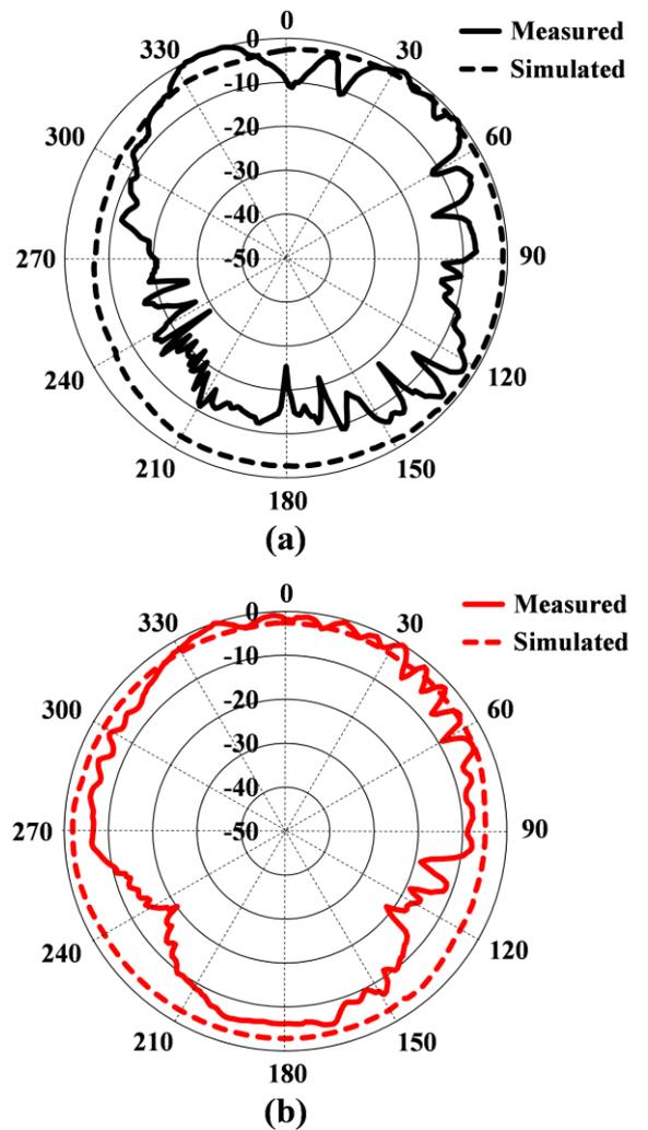
Fig. 9. The measured and simulated normalized gain pattern of the proposed CRLH antenna at frequency of 6 GHz, (a) x-z plane, and (b) y-z plane.
