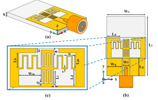
Fig. 2. Configuration of CRLH antenna (a) 3D layout (b) Top view, and (c) Zooming view for CRLH cell dimensions.
