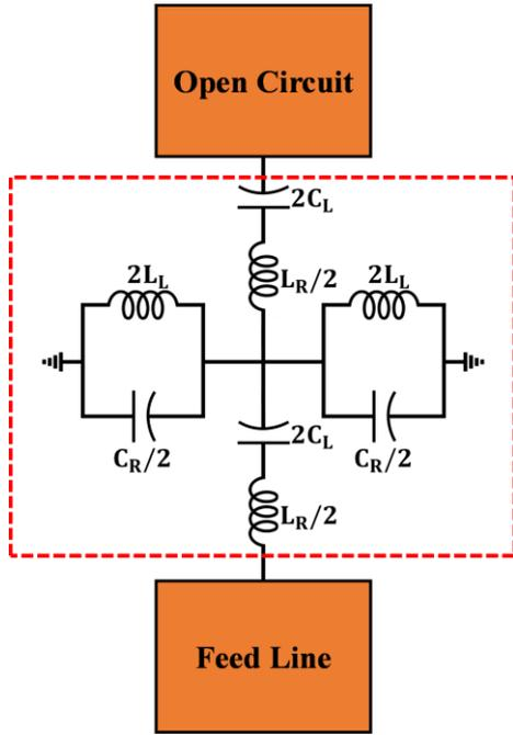
Fig. 3. The equivalent circuit model of the proposed CRLH antenna.
