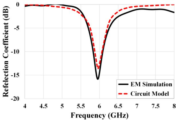
Fig. 4. The simulated reflection coefficient of the CRLH-antenna for the EM simulator and the equivalent circuit results.
