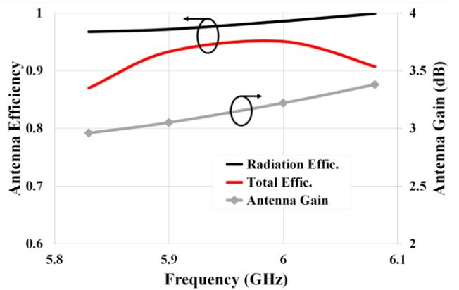
Fig. 6. The simulated gain and efficiencies of the proposed antenna at various values of frequency.
