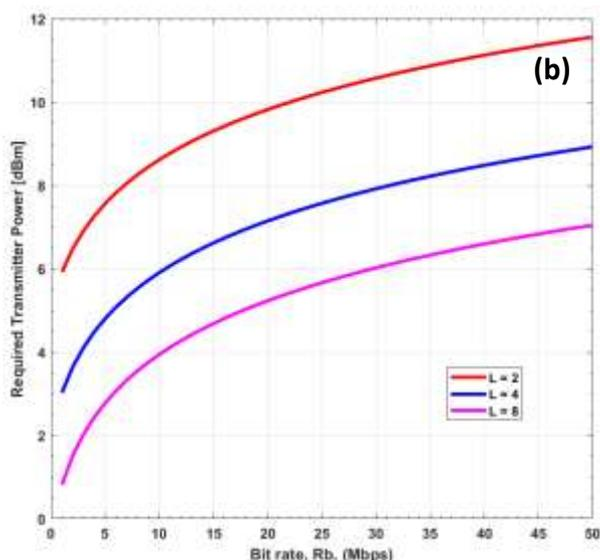
**Fig. 6** Minimum transmitter power required vs bit rate at different modulation levels (L) under distinctive lighting topology assumption for (a) without utilizing OFDM techniques, (b) by utilizing OFDM techniques.
