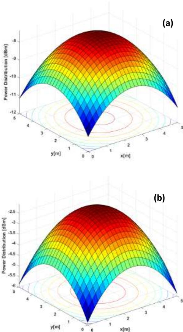
**Fig. 9** Power distribution across the proposed room under uniform lighting topology assumption for SC- LPPM (a) without utilizing OFDM techniques, (b) by utilizing OFDM techniques.
