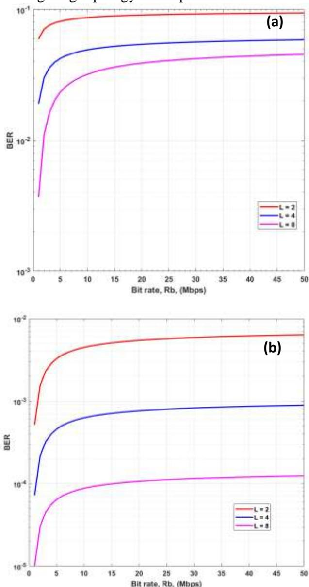
**Fig. 5** BER vs. bit rate at different modulation levels ( $L$ ) under uniform lighting topology assumption for (a) without utilizing OFDM techniques, (b) by utilizing OFDM techniques.
