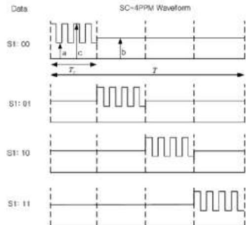
**Fig. 2.** SC-4 PPM waveform [21, 35].
