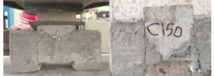
**Fig. 10. Failure at the interface**
