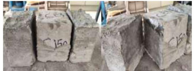
**Fig. 11. De-bonding in case of epoxy resin**
