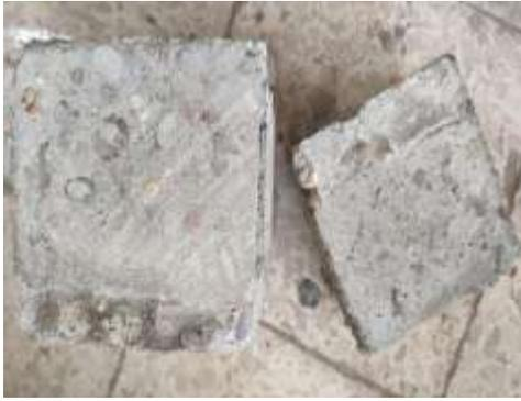
**Fig. 13. Interface failure without using any bonding agents**
