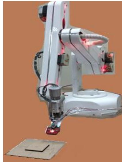
**Fig. 1:** ST arm robot with Takktile fingertip attached in end-effector.
