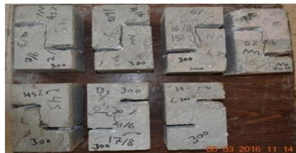
Figure (7) Patterns of cracks for specimens in category (Bs)
