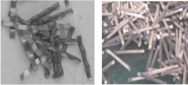
(a) Corrugated steel fiber. (b) Hooked end steel fiber.
