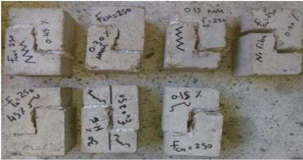
Figure (22): Pattern of cracks for category (Ar).
