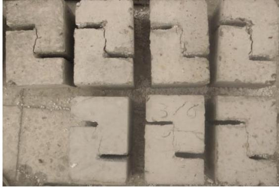
Figure (8) Patterns of cracks for specimens in category (Cs)
