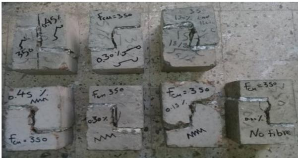
Figure (24): Pattern of cracks for category (Cr).
