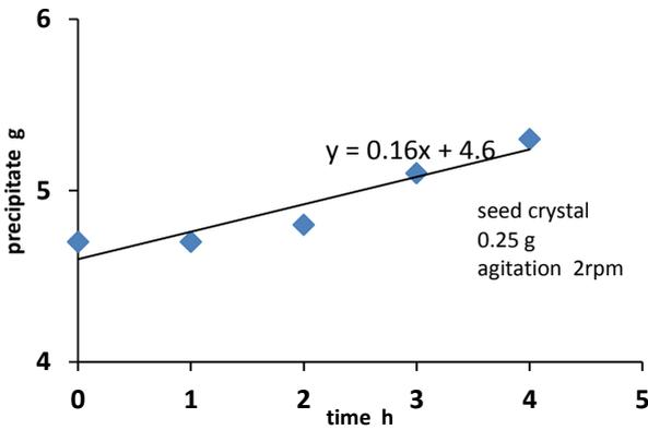
Fig. (6): precipitation without nano
