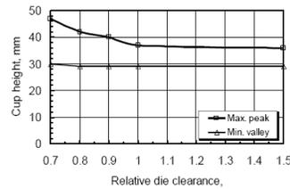
Figure 15. Variation of cup height versus relative die clearances of half hard aluminum cups ( $t_o = 1.91$  mm, BD=90 mm).
