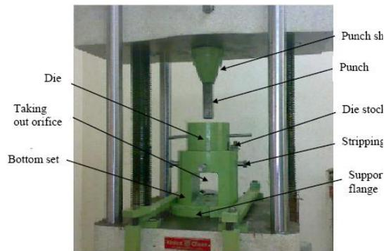
Figure1: Developed deep drawing apparatus.
