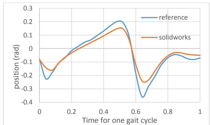
Figure 13: the reference position and position from CAD - CAM for the CSAAP.
