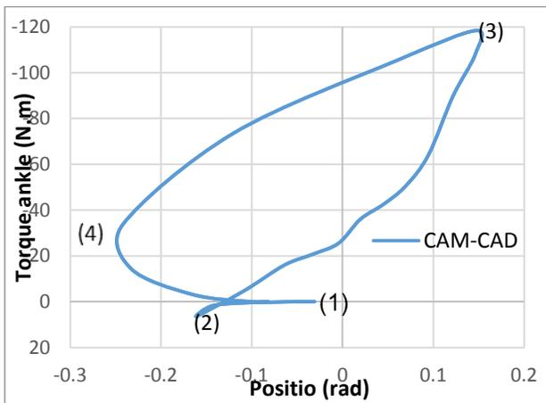
Figure 14: the angle-torque of the CSAAP for one gait period from CAD - CAM.
