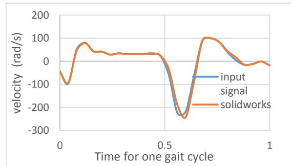
Figure 12: The input signal and the velocity of motor from CAD - CAM.
