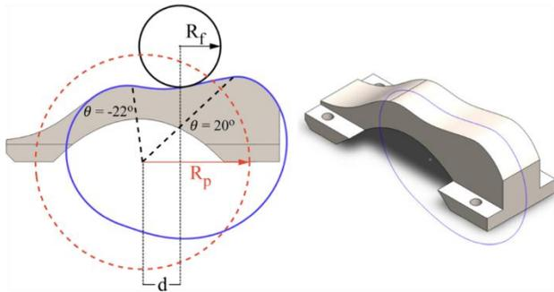
Figure 5: Cam prototype for SE+PEA mechanism.
