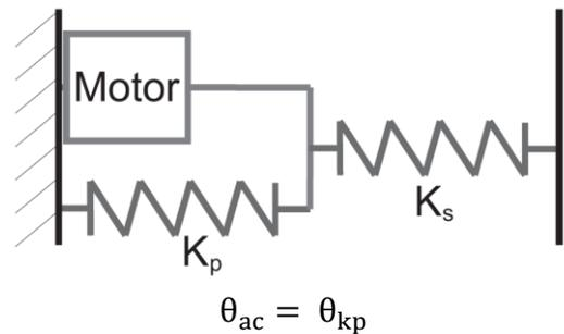
Figure 3: Schematic model of the Series Elastic and Parallel Elastic Actuator (SE+PEA)[29].
