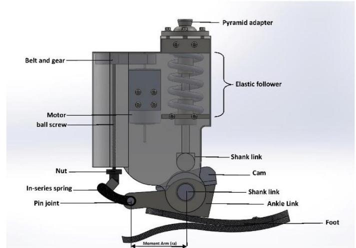
Figure 6: the model of the CSAAP in CAD - CAM program.
