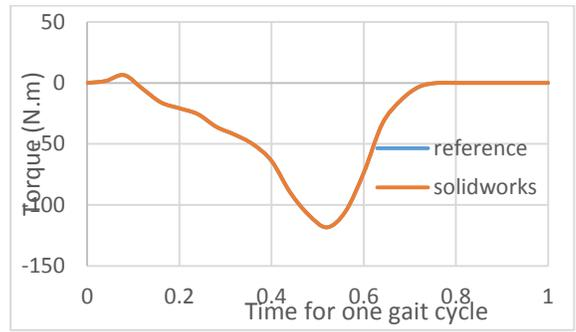
Figure 10: the reference torque for ankle and the torque for ankle from CAD - CAM.
