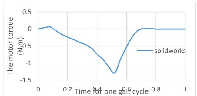
Figure 11: The torque for motor from CAD - CAM.
