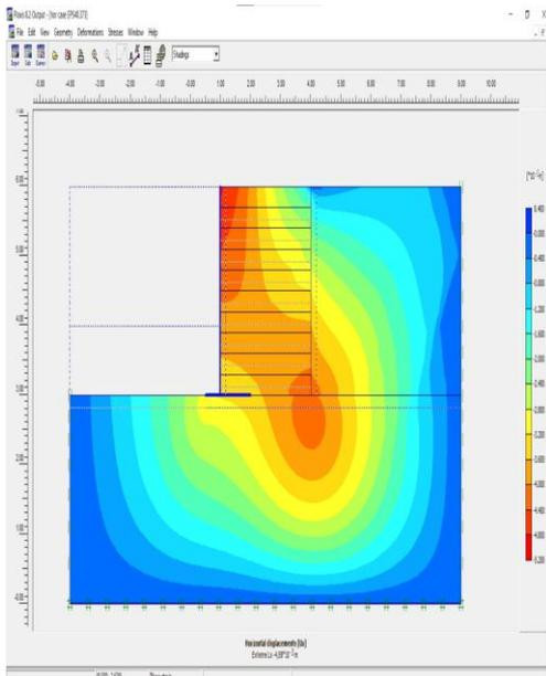
**Fig.8.** Horizontal displacement at final loop using EPS 40 for case III.
