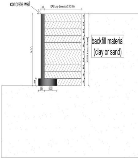
**Fig.2.** FE simulation with horizontally installation of geofoam.
