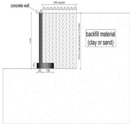
**Fig.3.** FE simulation with vertically installation of geofoam.
