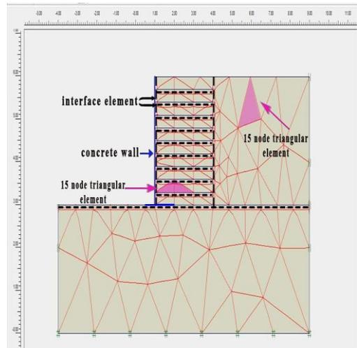
**Fig.4.** FE model mesh
