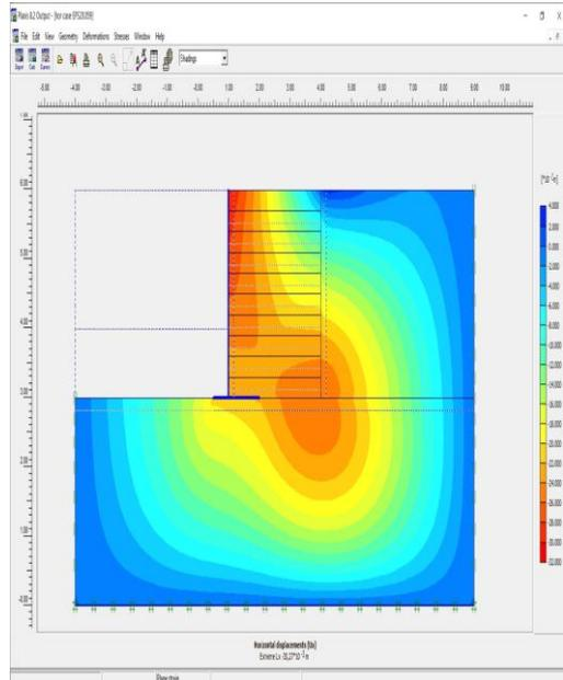
**Fig.6.** Horizontal displacement at final loop using EPS 20 for case I.
